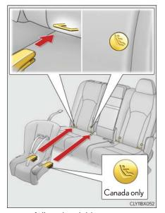
If the child restraint has a top tether strap, follow the child restraint manufacturer's operation manual regarding the installation, using the top tether strap to latch onto the top tether strap anchor.  $(\rightarrow P. 70)$
