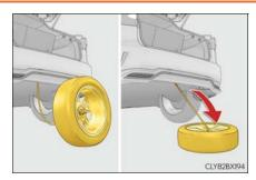
before raising the tire, make sure that the hoist assembly is perpendicular to the wheel opening. (Try to place the tire directly beneath the vehicle, near where the wire cable is hanging from.)
