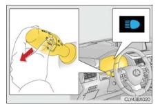
**2** Press the Automatic High Beam switch.
