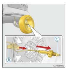
3 Fully depress the secondary latch (A) and install the bracket (B) to the hoist assembly ©.
