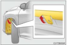
3 Partially remove the fender liner and turn the bulb base counter-clockwise and remove it.
