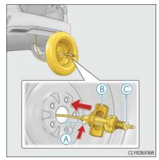
8 Tilt the bracket B and pass it through the wheel opening. Then remove the hoist assembly ©.
