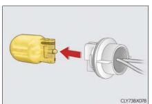
After installing the bulb base, wiggle it lightly to make sure it is securely installed and turn on the rear turn signal lights to visually check that there is no light leaking from between the bulb base and light unit.
