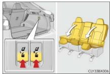
When using the seatback angle adjustment switch: If the rear seatback is reclined, adjust it to the most upright position and then press the switch again.
