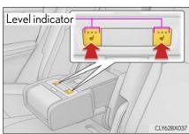
Each time the switch is pressed, the operation condition changes as follows. Hi (3 segments lit)  $\rightarrow$  Mid (2 segments lit)  $\rightarrow$  Lo (1 segment lit)  $\rightarrow$  Off
