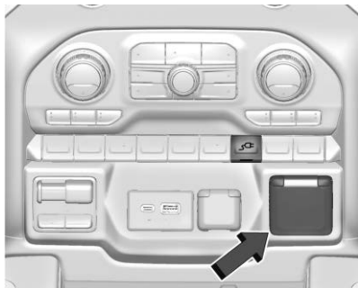
In Cab Power Outlet and DC/AC Switch
