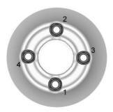
Tighten the wheel nuts firmly with the wheel wrench in a crisscross sequence, as shown
