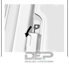
To open the fuel filler door, lift the fuel door release lever. The lever is on the floor, on the left front side of the driver seat. The fuel door is unlocked when the vehicle is unlocked. Locking the vehicle locks the fuel door.
