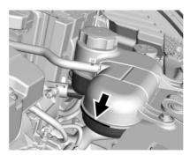
Check to see if coolant is visible in the coolant surge tank. If the coolant inside the coolant surge tank is
