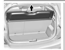
To remove, pull the cargo cover upward.
