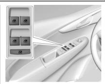
Power windows work when the ignition is on, in ACC/ACCESSORY, or when Retained Accessory Power (RAP) is active. See Retained Accessory Power (RAP)
