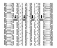
Treadwear indicators are one way to tell when it is time for new tires. Treadwear indicators appear when the tires have only 1.6 mm (1/16 in) or less of tread remaining. See *Tire Inspection*  $\Rightarrow$  259 and *Tire Rotation*  $\Rightarrow$  259.
