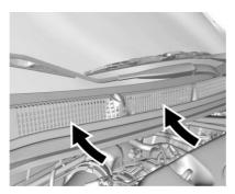
The air intake at the base of the windshield under the hood must be kept clear to allow the flow of air into the vehicle. Clear away any ice, snow, or leaves.
