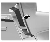
Move the seat belt out of the way by putting the seat belts into the belt guide on the trim. The seat belt should not cross the seatback locking mechanism when raising the seatback.
