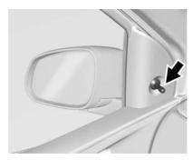
If equipped, controls for the outside manual mirrors are next to each mirror. Adjust to see a little of the side of the vehicle.
