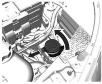
For the driver side bulb, remove the washer funnel by turning it counterclockwise and pulling it straight out.
