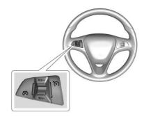
(S): Press to turn the cruise control system on and off. A white indicator comes on in the instrument cluster when cruise is turned on.
