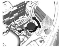
Remove the washer funnel by turning it counterclockwise and pulling it straight out.
