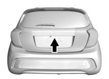
Press the touch pad and lift to open or, if equipped, pull the handle and lift up.
