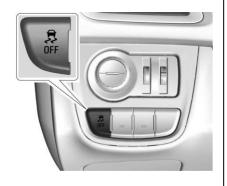
The button for TCS and StabiliTrak/ ESC is on the lower instrument panel to the left of the steering wheel.
