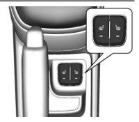
If equipped, the buttons are on the center console. To operate, the engine must be running.
