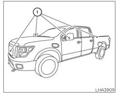
If dirt, rain or snow accumulates on any of the cameras ①, the MOD system may not operate properly. Clean the camera by wiping with a cloth dampened with a diluted mild cleaning agent and then wiping with a dry cloth.
