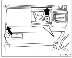
The extended storage switch is used when shipping the vehicle. It is located in the fuse panel inside the glove box. To reach it, open the glove box ① on the instrument panel, then open the fuse panel cover ②.
