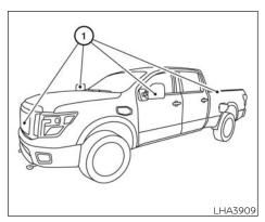
If dirt, rain or snow accumulates on any of the cameras (1), the Intelligent Around View Monitor may not display objects clearly. Clean the camera by wiping with a cloth dampened with a diluted mild cleaning agent and then wiping with a dry cloth.
