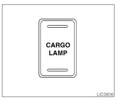
To turn on the cargo lamp and the under rail bed lamps (if so equipped) push the switch down to the ON position. The tailgate lights (if so equipped) will also illuminate when the cargo lamp switch is in the ON position.
