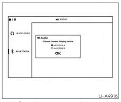
audio from the Passenger side monitor. Select OK to confirm and store the desired monitor
