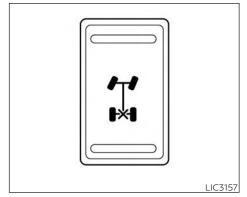
The E-Lock system can help provide added traction if the vehicle is stuck or becoming stuck.
