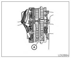
5. Remove the fuse with the fuse puller
