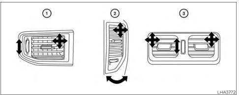
Adjust air flow direction for the driver's and passenger's side vents (1), center vents (2). and rear passengers' vents (if so equipped) (3) by moving the vent slide and/or vent assemblies
