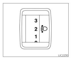
Manual headlight aiming control (if so equipped)
