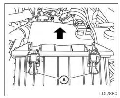
The dry paper type filter element may be cleaned and reused. Replace it according to the maintenance log shown in the Titan Owner's Manual.
