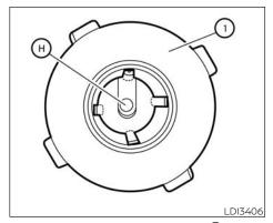
10. Inspect the fuel filter element ① for the No Filter No Run (NFNR) pin ① and replace fuel filter element if pin is damaged or missing.
