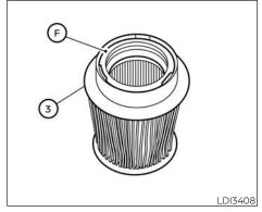
9. Inspect the fuel filter element (Stage 2 3) to verify the inner seal (F) is present. If inner seal is missing from the filter element proceed to step 10.
