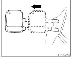
Pull the trailer tow mirror outward to extend it to the desired position for better visibility while towing a trailer.
