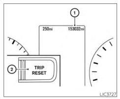
Odometer/Twin trip odometer
