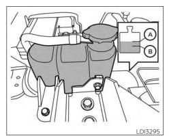
VK56VD engine (non-XD model) CHECKING ENGINE COOLANT I FVFI
