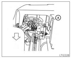
3. Locate the jumper harness connector under the lower portion of the instrument panel. The connector is taped to the wiring harness (A) as indicated.
