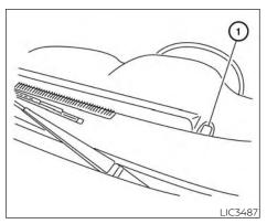
Be sure you do not put anything on top of the autolight sensor (1) located on the top side of the instrument panel. The autolight sensor controls the autolight; if it is covered, the autolight sensor reacts as if it is dark out and the headlights will illuminate. If this occurs while parked with the engine off and the ignition switch placed in the ON position, your vehicle's battery could become discharged.
