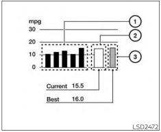
When the ignition switch is in the OFF position, the ECO management display appears.
