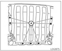
Skid plate (Type B) (if so equipped)
