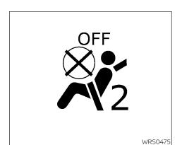
7. If the booster seat is installed in the front passenger seat, place the ignition switch in the ON position. The front passenger air bag status light 🌋 equipped) may or may not illuminate, depending on the size of the child and the type of booster seat being used. For additional information, refer to "Front passenger air bag and status light" in this section
