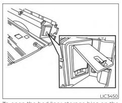
To open the bed liner storage bins on the tail gate end of the bed liner, lift the tab away from the truck bed, pull the lid up and away from the truck.
