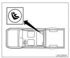
**LATCH** system lower anchor locations LATCH (Lower Anchors and Tethers for CHildren) SYSTEM (Crew Cab models and King Cab® models with rear bench seat)
