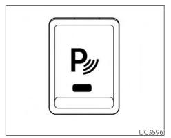
The Front and rear sonar system OFF switch on the instrument panel allows the driver to turn the Front and rear sonar system, Moving Object Detection (MOD) (if so equipped), and Rear Cross Traffic Alert (RCTA) system on and off. To turn the systems on and off, the ignition switch must be in the ON position.
