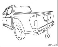
If dirt, rain or snow accumulates on the camera (1), the RearView Monitor may not display objects clearly. Clean the camera by wiping it with a cloth dampened with a diluted mild cleaning agent and then wiping it with a dry cloth.
