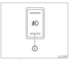
To turn the fog lights on, turn the headlight switch to the  $\mathfrak{D}$  position, then push the fog light switch  $\mathfrak{I}$  on.
