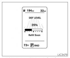
DIESEL EXHAUST FLUID (DEF) LEVEL (if so equipped)
