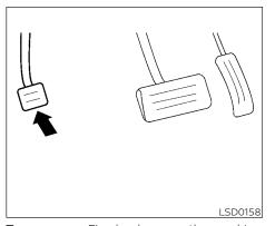
To engage: Firmly depress the parking brake
