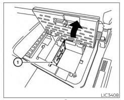
To adjust the divider ①, pull it straight up and reposition it to the desired location, sliding it straight down.
