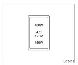
To use the outlets for devices that require 120v power, place the ignition in the ON position and push the power inverter switch
