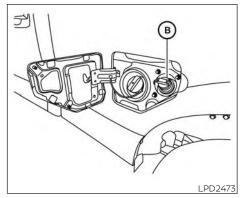
DEF will freeze below 12°F (-11°C); however, your vehicle is equipped with an automatic preheating system, which allows the DEF system to operate below 12°F (-11°C). When the vehicle is not in operation for an extended period of time with temperatures at or below 12°F (-11°C), the DEF tank could freeze. In this condition, adding DEF will not change the gauge level and added DEF will not reach the pump, because it will sit on top of the frozen layer.
