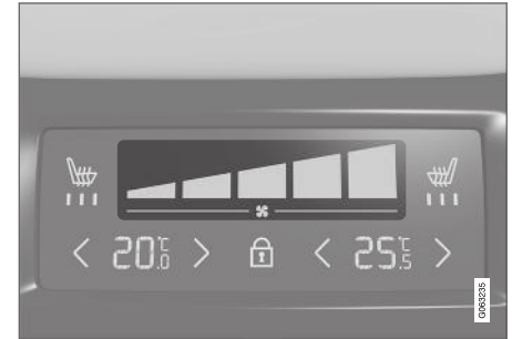
Blower controls on the rear climate panel of the tunnel console.
