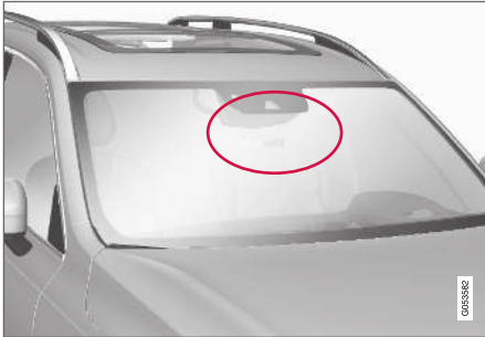
The area marked in the illustration must be kept free of decals, objects, solar film, etc. 63
