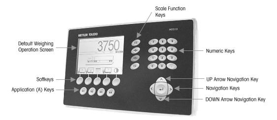
Figure 2-1: Key Locations and Default Weighing Operation Screen
