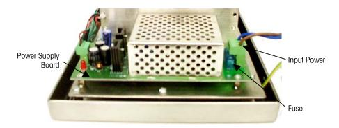
Figure A-5: Power Supply Board
