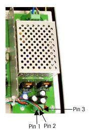
Figure 4-1: Pins 1, 2, and 3 on the Power Supply Board
