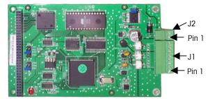
Figure A-9: POWERCELL Board Connector Locations
