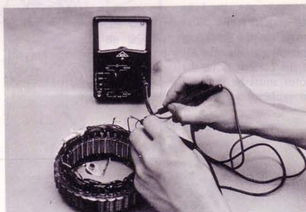
Fig. 5-19 Checking stator coil for open
