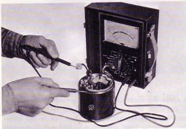
Fig. 5-40 Checking field coil for ground
