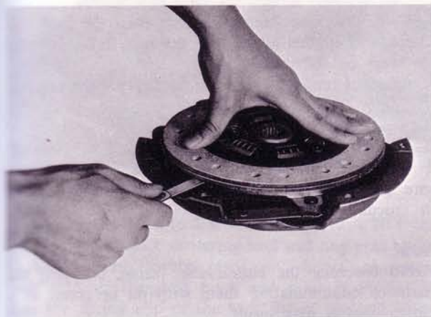
Fig. 6-5 Checking clutch disc for warpage
