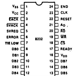
Figure 2. Pin Configuration
