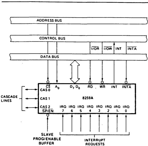
Figure 1. 8259A Interface to Standard System Bus
