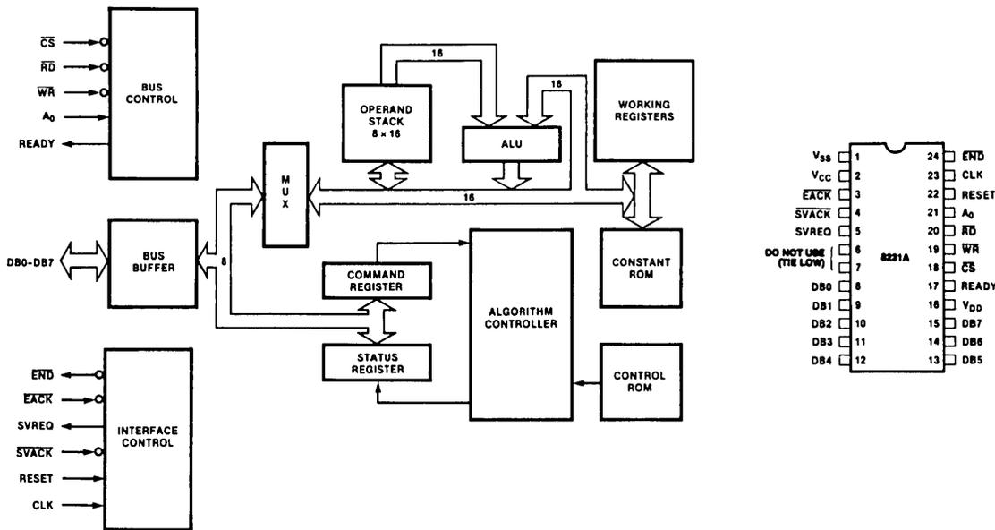
Figure 1. Block Diagram
