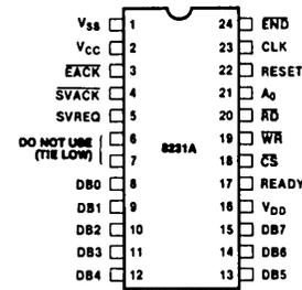
Figure 2. Pin Configuration
