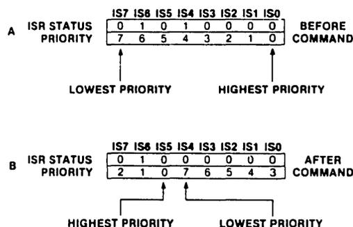
Figure 13. A-B. Rotate on Non-specific EOI Command Example
