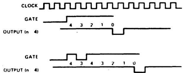
Figure 5. 8253 Timing Diagrams
