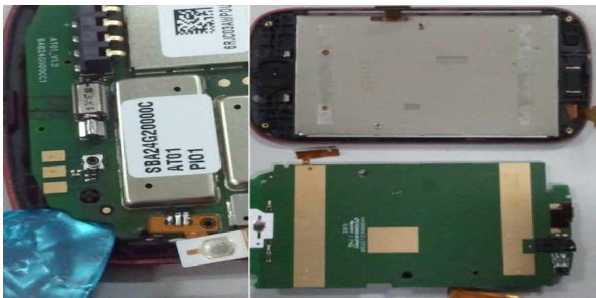
Step 7: Separate FPC from the PCBA(Temperature: 350 \pm 10^{\circ}\text{C} )
