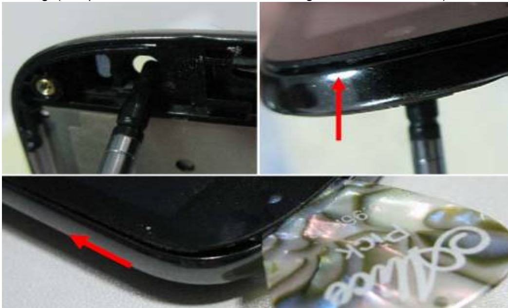
Step 8: Firstly, Please use hot wind gun heating around the touch lens, then separate the touch lens from furnished front casing. (Temperature: 100±10°C, Air Level:3, Height:5-10mm, Time:30s)
