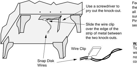
Feed the two snap disk wires into the eye of the wire clip. Remove all slack from the wire, making sure not to dislodge the snap disk. Pinch the eye of the wire clip to secure the wires.
