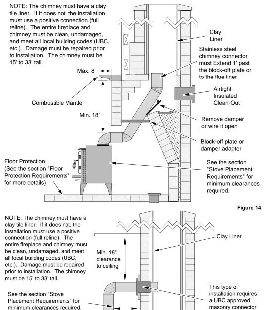
Interior or Exterior Masonry Chimney
