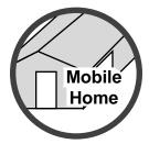
When installed in a mobile home, this appliance must be bolted to the floor, have outside air, and not be installed in the bedroom (Per H.U.D. requirements). Check with local building officials.
