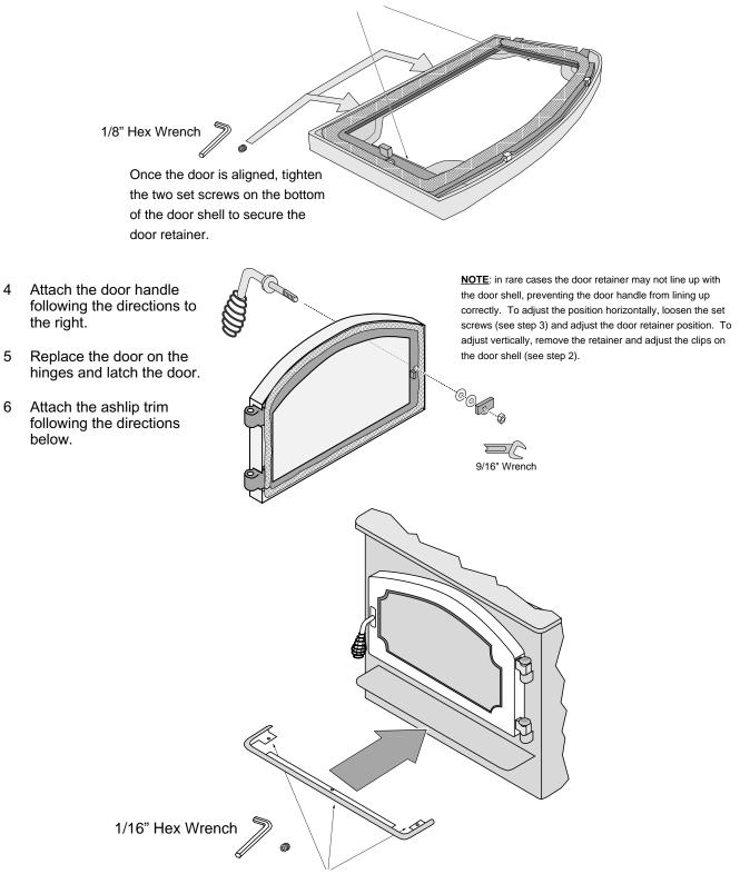
Slide the ashlip trim into place then tighten the three set screws on the bottom of the ashlip to secure.
