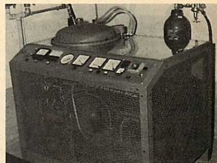
Fig. 3—The diamond tips are bonded to the sapphire shanks in this controlled atmosphere furnace.
