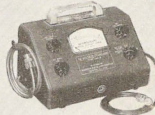
RF VOLTAGE STANDARD TYPE 245-A
