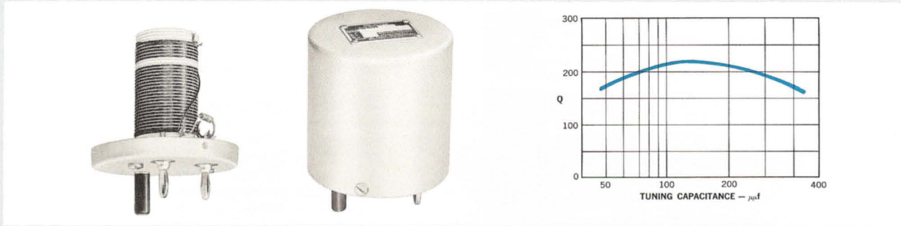
Illustrating construction, also relationship between Q and tuning capacitance for typical inductor
