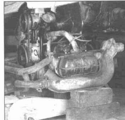
12.23b Let the engine down on blocks positioned under both heat exchangers
