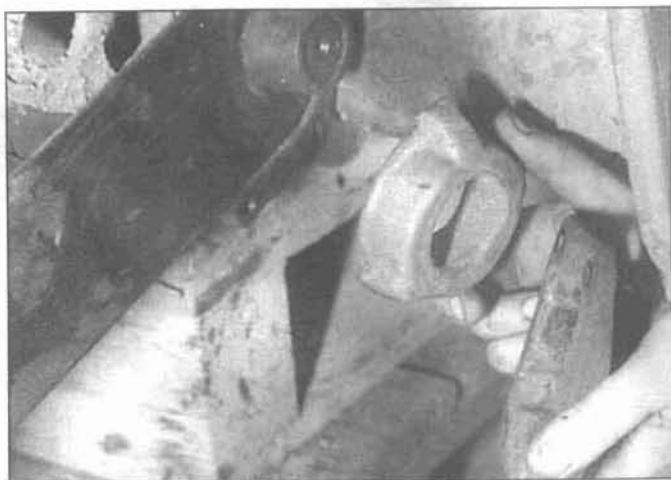
13.9b Remove the rubber bushing from the hub
