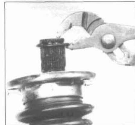
12.8a Remove the concave washer by working it up the shaft with pliers
