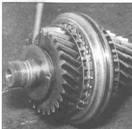
9.47a Install the thrust washer on the end of the input shaft with the V-cuts facing the front of the shaft
