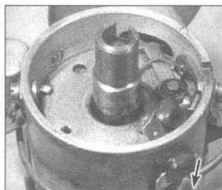
27.6 If the points are mounted externally like this, remove the screw (arrow) and pull the connector block out of the housing
