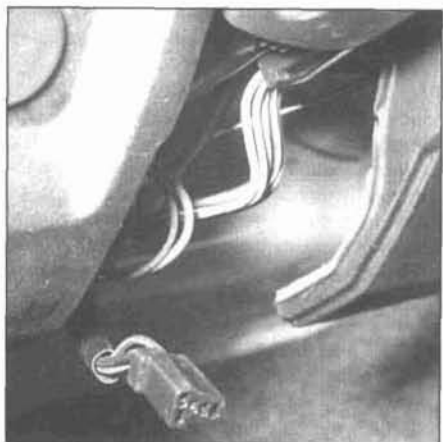
15.18b ... and unplug the electrical connector under the steering column
