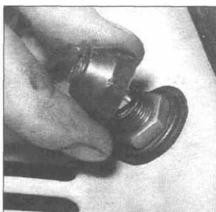
15.15a Remove the wiper shaft covers ...
