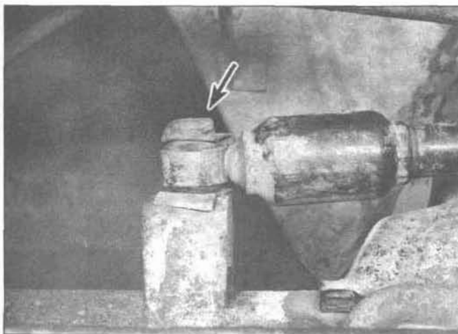
17.2b Remove the bolt (arrow) that attaches the steering damper to its mounting bracket on the upper axle tube
