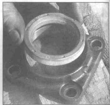
8.10 Place the bearing cover on a block of wood, position the new seal - numbers facing up, open side facing down - square with the recessed bore in the cover and carefully tap the seal into place
