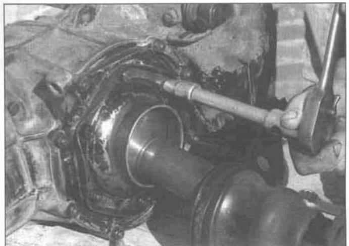
10.6a Remove the six nuts on the axle tube retainer
