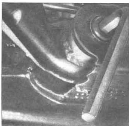
15.9 Remove the Allen pivot bolt from the front end of the diagonal arm
