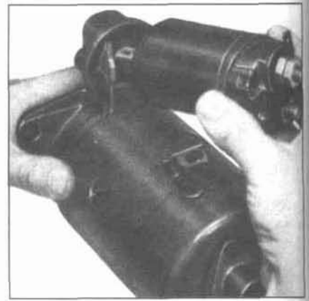
17.5 Lift the solenoid free of the starter (Bosch shown)
