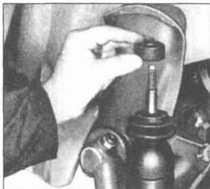
2.7b Install the damping ring on the shock absorber before you slip the damper rod through the upper mounting hole in the shock tower
