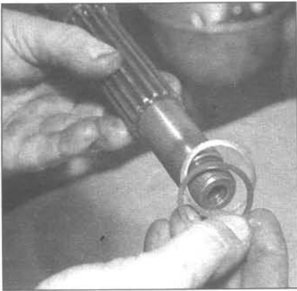
7.38a Install the same number of shims, in the same order, that you removed from the pinion shaft
