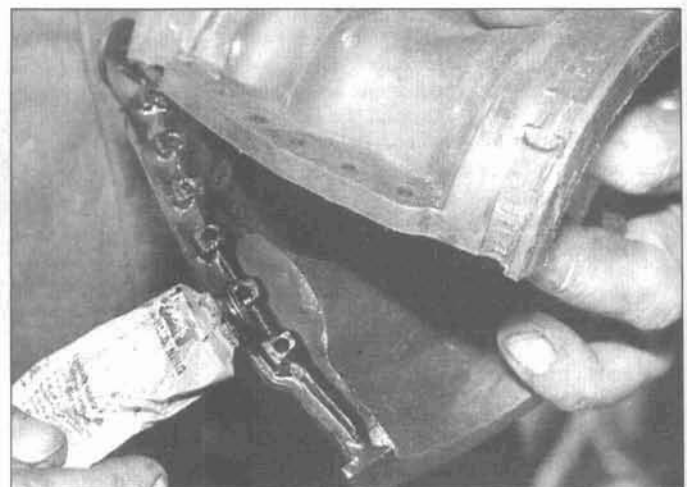
9.4 Apply a thin coat of sealing compound to the mating surfaces of the boot
