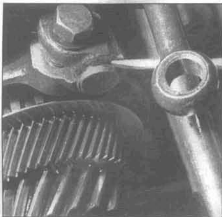
9.68c This is how the third/fourth selector fork looks when it's properly positioned
