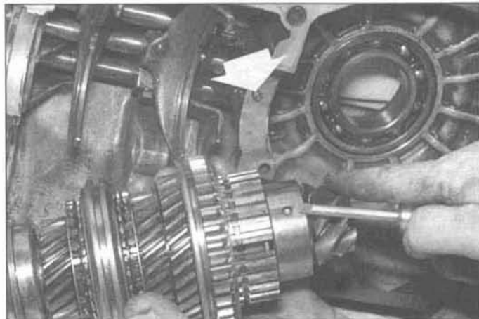
7.57a To check the setting of the selector forks, temporarily place the assembled pinion shaft in position in the left case half (note the locating dowel (arrow) for the bearing) . . .
