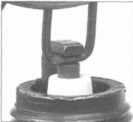
25.4a Spark plug manufacturers recommend using a wire-type gauge when checking the gap - if the wire does not slide between the electrodes with a slight drag, adjustment is required
