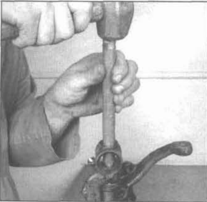
5.16 Drive the old kingpin out of the carrier and knuckle with a hammer and punch (if you can't drive them out, they'll have to be removed with a hydraulic press)
