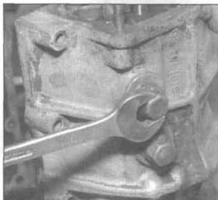
8.4a If third gear jumps out, remove the front plug from the transaxle . . .
