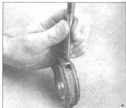
23.12a Mark the cylinder number on the rods with a sharp punch - two dots for number two cylinder, etc.
