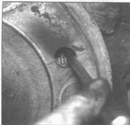
2.3a If the front brake drum is binding on the brake shoes, insert a screwdriver through the adjustment hole in the drum, turn the adjuster until the shoes are no longer binding . . .
