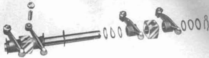
3.6a 1965 and earlier rocker arm assembly - exploded view
