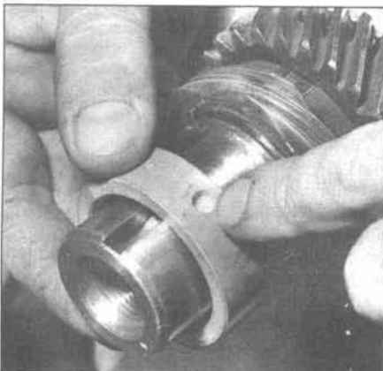
30.6 Install the number four bearing with the offset hole toward the flywheel end
