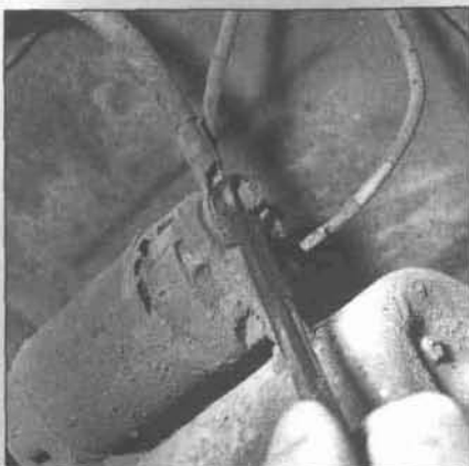
16.3 Unplug the small wires and remove the nut from the solenoid, then detach the battery cable
