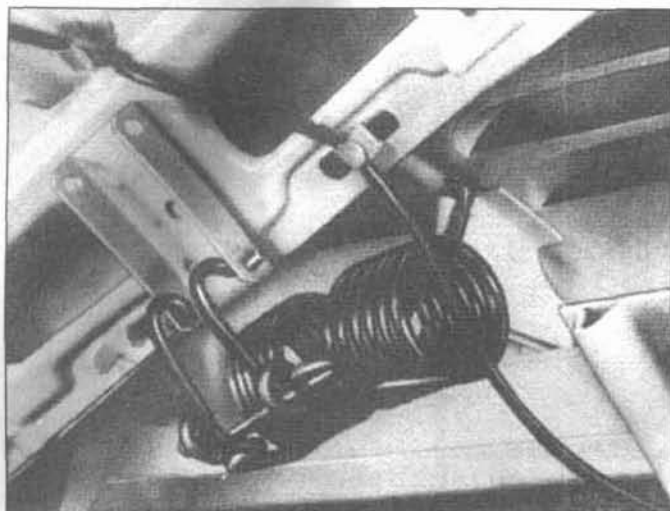
11.4 Lift the hood off its hinge brackets so the spring can unhook from the bracket on the roof panel
