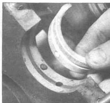
32.5a Align the hole in the bearing with the dowel
