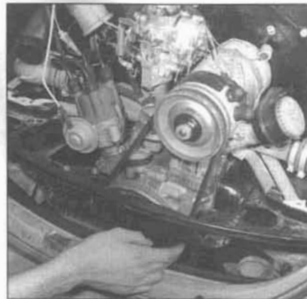
12.11c . . . and detach the rear cover
