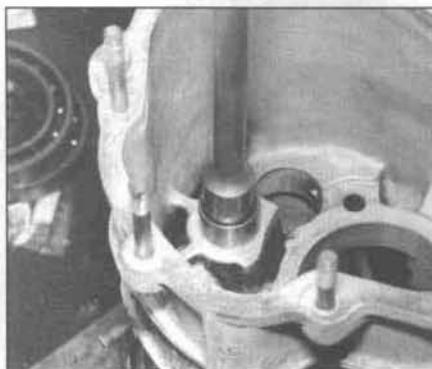
9.62b Drive one cage into the case with a socket on an extension so that it's flush with the one end of the bore - the metal face of the end of the needle should face in ...
