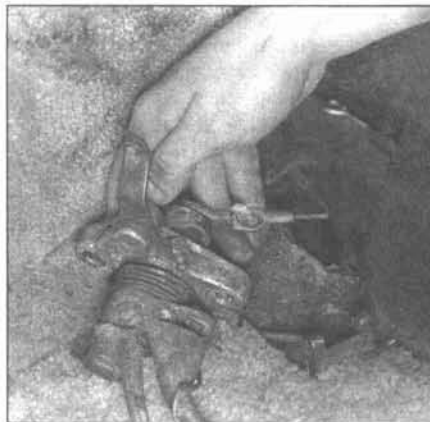
3.6 Pull out the pedal cluster and disconnect the clutch cable from the clutch pedal shaft
