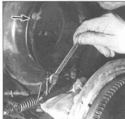
2.3b The rubber pad (arrow) should just touch the fan shroud when the engine is cold - be sure the mounting bolts are tight (engine removed for clarity)
