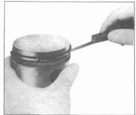
22.10 Check the ring side clearance with a feeler gauge at several points around the groove
