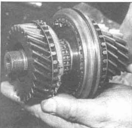
9.46c ... and install the synchro ring and fourth gear
