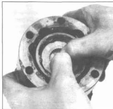
12.7 Hold the CV joint securely and push the axle shaft out with your thumbs
