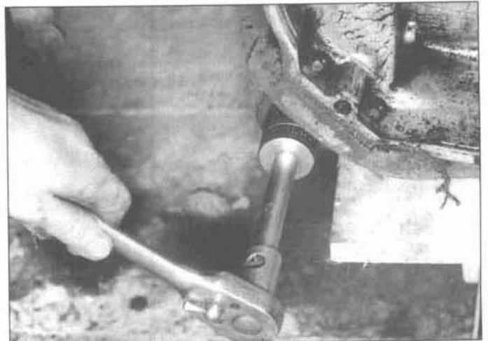
5.19 Remove the transaxle carrier bolts
