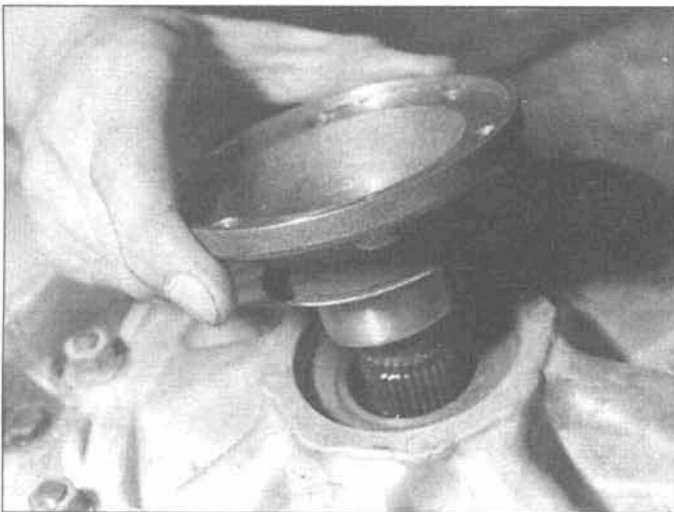
9.100b . . . push the drive flange onto the shaft . . .
