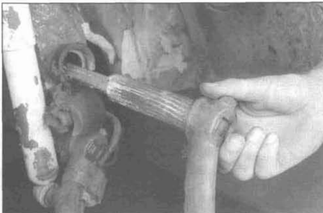
8.6 Use one of the torsion arms to pull the torsion bars out of the axle tube
