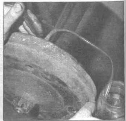
9.7 When bleeding the brakes, a hose is connected to the bleeder valve at the wheel cylinder (or caliper) and then submerged in brake fluid - air will be seen as bubbles in the hose and container when the pedal is depressed and the bleeder valve is opened
