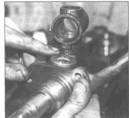
5.19b . . . make sure the dimples in the cover and washers are aligned with the dowel in the knuckle
