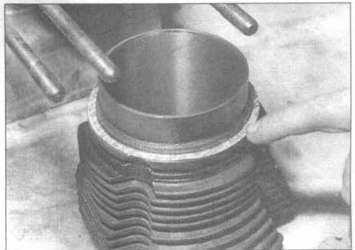
34.2 Put a new gasket on the base of the cylinder
