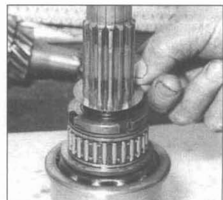
9.49 Install the thrust shim(s) on the pinion shaft that control first gear endplay
