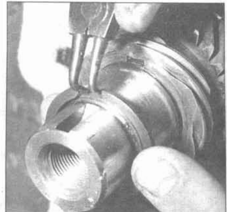
30.5 Install the circlip in the groove next to the distributor drive gear
