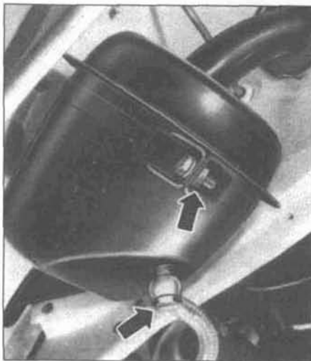
10.4 Typical ATF tank assembly (Beetle shown) - to remove it, disconnect the ATF suction line fitting (lower arrow), take off the nuts attaching the trim plate to the quarter panel (see illustration 10.2) and remove the strap bolt
