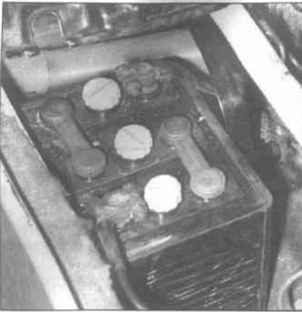
4.7a Six-volt batteries have three caps
