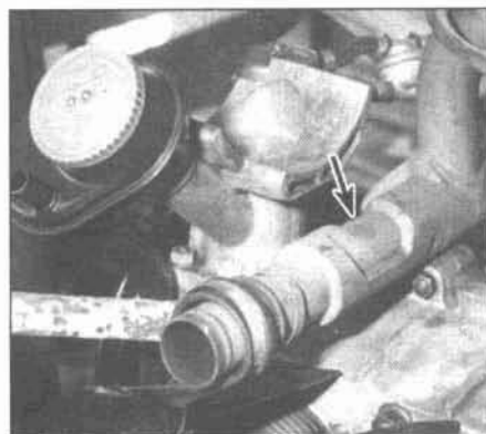
4.13 Remove the nut (arrow) and lift the manifold center section from the engine
