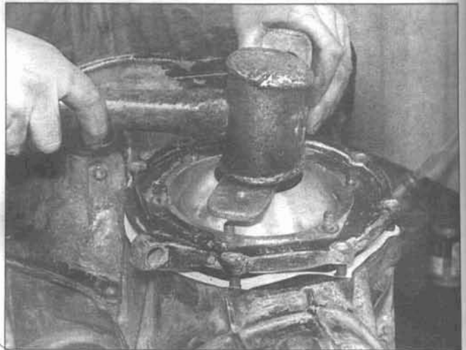
9.98b Carefully tap the left bearing side cover down onto the differential - don't use the retaining nuts to draw it down or you may crack the cover
