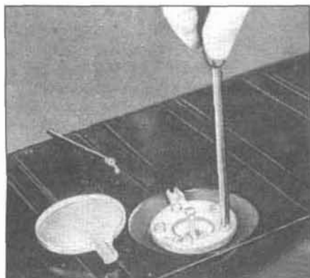
14.7 To remove the mechanical fuel gauge sending unit, remove the cover, disconnect the cable or wire to the gauge and remove the flange mounting screws
