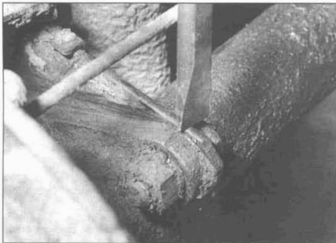
13.4 On swing axle models, mark the spring plate position in relation to the housing for the rear axle bearing
