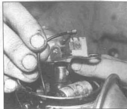
27.5b On some early models, the wire connector is attached with a screw
