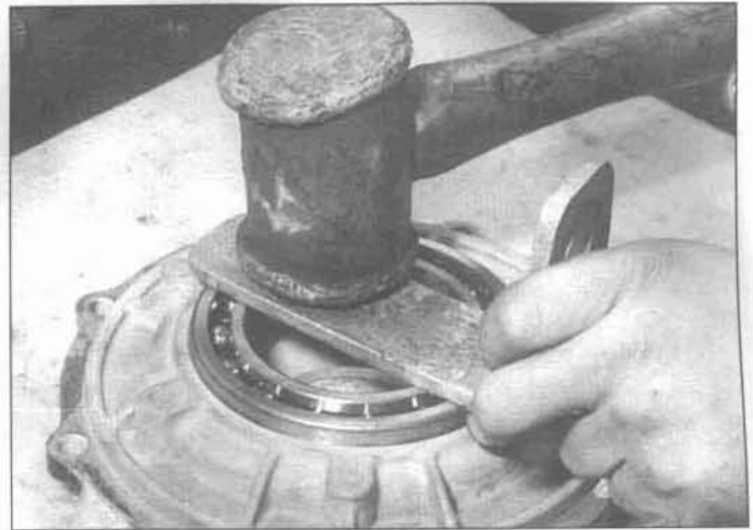
9.93 To install new side bearings, support the side cover evenly and securely, then tap the new bearing into place with a wide, flat metal bar or a block of wood - the closed side of the ball race must face toward the outside of the case
