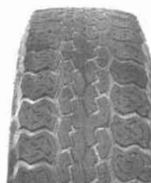
FEATHERING DUE TO MISALIGNMENT
