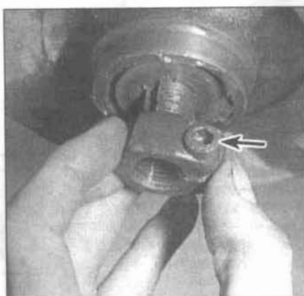
32.8 Loosen the lock bolt (arrow) and back the nut off
