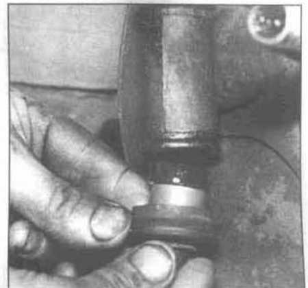
2.3i Even if the wheel cylinder doesn't appear to be leaking, it's a good idea to pull the pistons and seals out and inspect them while the brake is disassembled - if they're rusted, pitted or scored, replace or rebuild the wheel cylinder (see Section 3)
