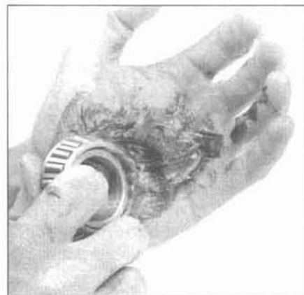
32.15 Work grease into the bearing rollers by pressing it against the palm of your hand
