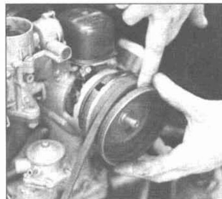
18.6a Hold the belt in place as you install the outer pulley
