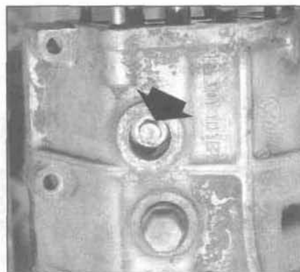
8.4b . . . loosen the selector fork set screw, slide the fork to the rear on its rail, tighten the set screw, install the plug and road test the vehicle to check your work - you may have to repeat this process several times until the gear mesh feels right
