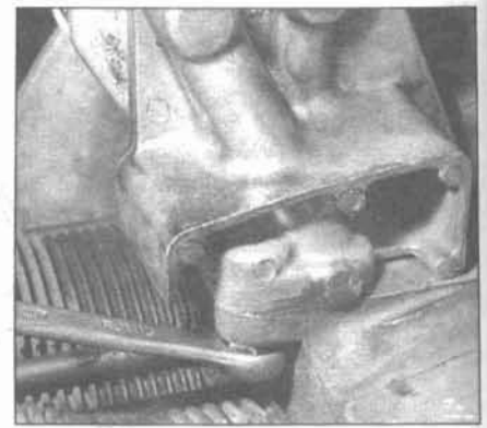
5.5 Remove the adapter from the engine (1971 and later models)
