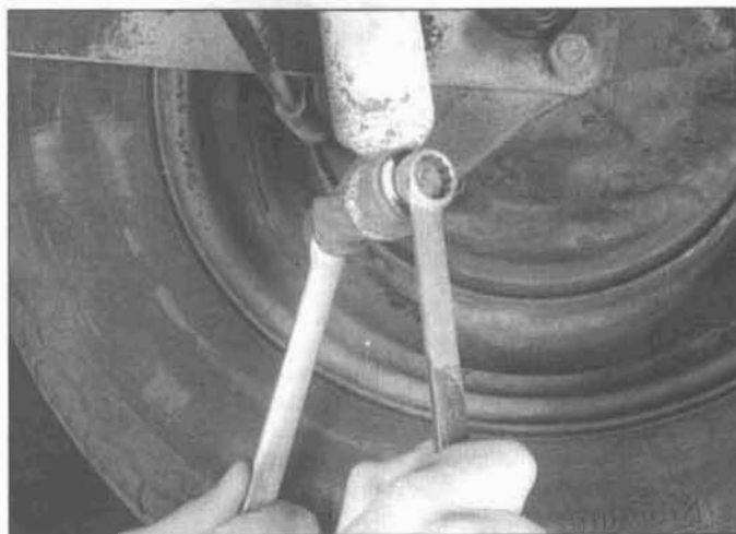
12.2b Lower shock mounting bolt and nut
