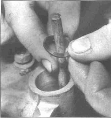
8.10 Slide the shims down the rod
