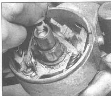
27.5a Disconnect the wire from the points at the terminal
