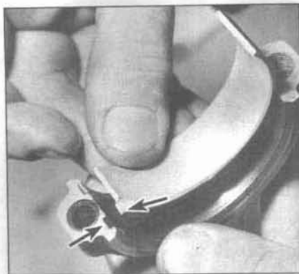
31.2 The bearing tang must engage the notch (arrows)
