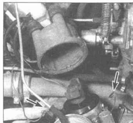
26.11a Pop the two retaining clips (arrows) off and lift the cap
