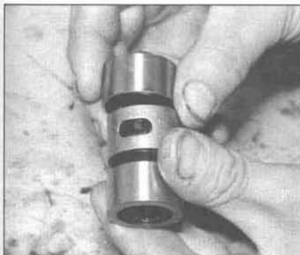
9.62a The needle roller bearings for the reverse drive shaft consists of two roller cages and a spacer between them
