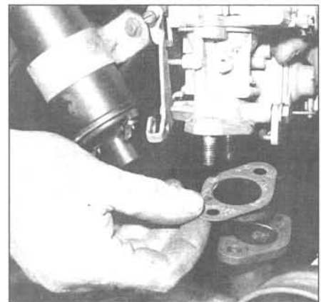
9.9 Place a new gasket between the carburetor and intake manifold
