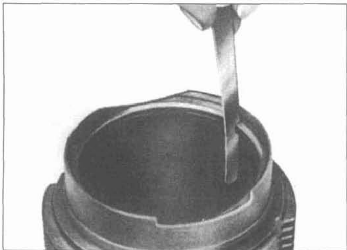
33.4 Insert each ring into the cylinder and measure the end gap with a feeler gauge
