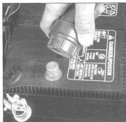
6.7a Regardless of the type of tool used on the battery posts, a clean, shiny surface should be the result
