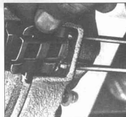
4.17b . . . and pull the retaining pin out of the caliper housing
