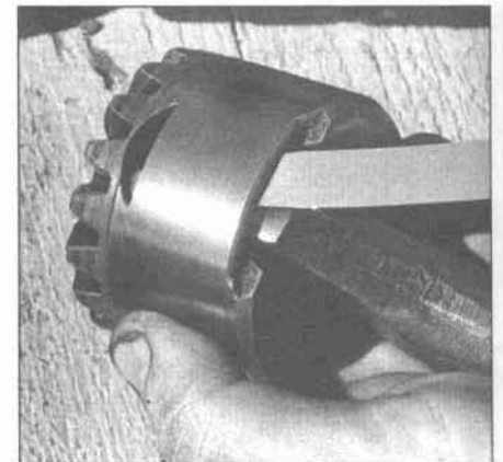
10.17 Using a feeler gauge of the correct thickness, measure the thickness between the rounded ends of the flat-bladed tip of the axle shaft and the inner diameter of the differential side gear
