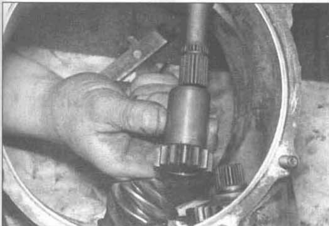
9.87a Install the reverse gear/splined sleeve onto the shaft, plain end first . . .
