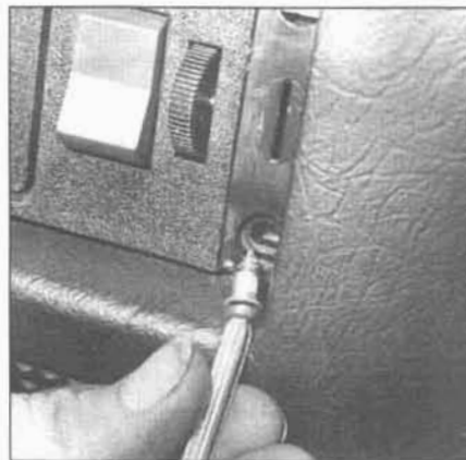
10.12 Remove these sheet metal screws from each end of the instrument panel switch cluster
