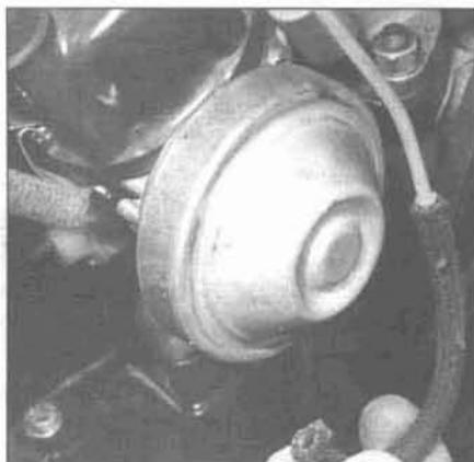
8.4 Disconnect the vacuum hose(s) from the distributor - if there are two hoses, label them
