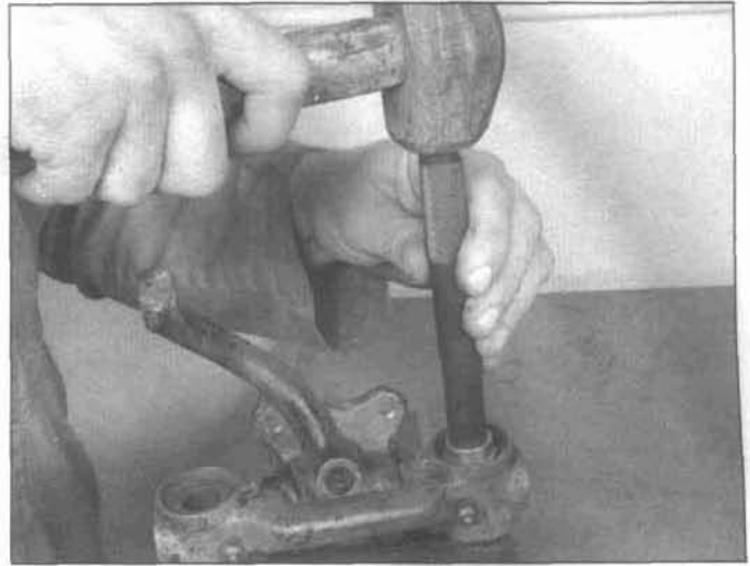
5.15 Drive the old linkpin bushings out of the carrier
