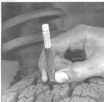
5.2 Use a tire tread depth indicator to monitor tire wear - they are available at auto parts stores and service stations and cost very little
