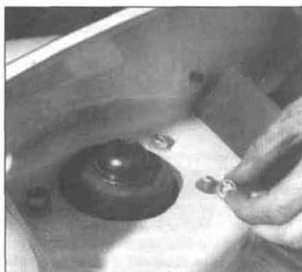
3.7 Working from inside the luggage compartment, remove these three upper mounting nuts - when you get to the third nut, reach under the fender and hold the strut so it doesn't fall when you remove the nut
