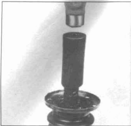
12.17 Use a hammer and deep socket to tap on the concave washer until it's at the base of the splines
