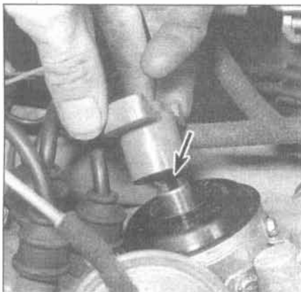
26.12a Pull the rotor straight up - note the notch in the distributor shaft (arrow) must align with the tab in the rotors
