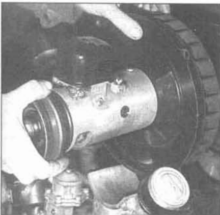
12.6 Lift the generator from the fan housing
