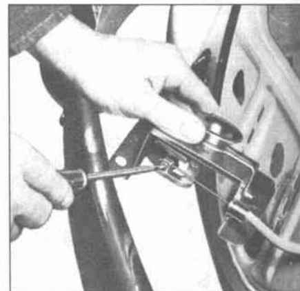
10.3 . . . pull out the lock, loosen the clamping screw and detach the cable
