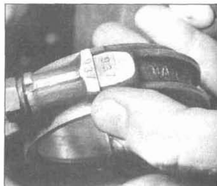
23.12b The rods have numbers such as this on them - be sure they are kept together
