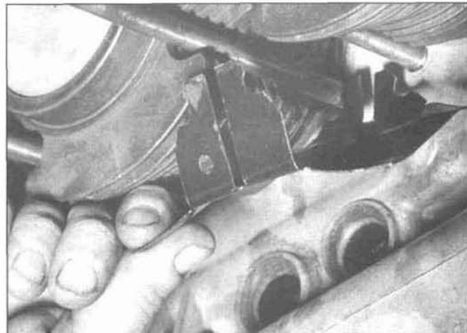
34.11 Install the air deflector plates between the cylinders on the underside (engine mounted on stand and turned upside-down for ease of installation)
