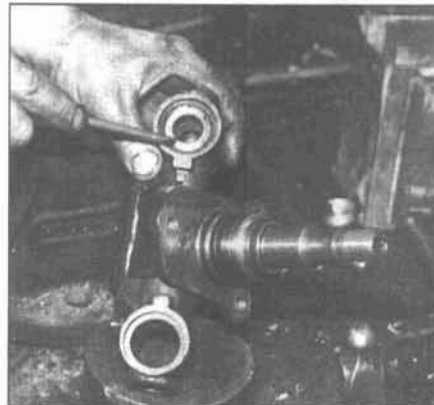
5.21c The linkpin bushings should be flush with the end of the carrier when installed
