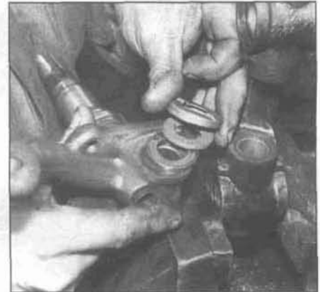
5.19a When you install the new steel thrust washer, plastic thrust washer and thrust washer cover . . .
