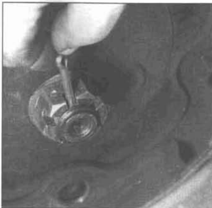
2.3k To begin the rear brake shoe replacement procedure, remove the cotter pin from the castle nut on the rear axle
