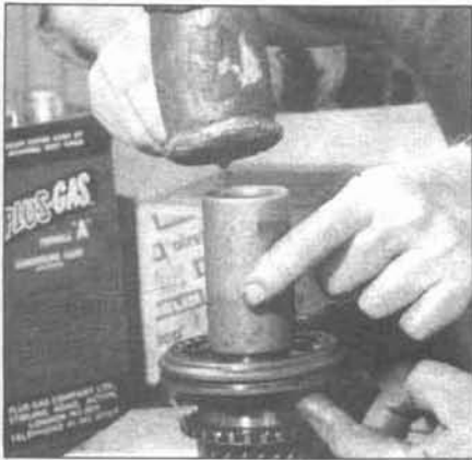
9.45c ... then drive on the hub with a suitable piece of pipe and a heavy hammer
