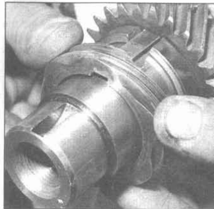
30.4 Carefully guide the distributor drive gear onto the crankshaft
