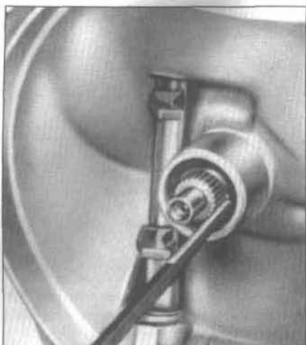
8.24 Using a small hook-type seal puller, dig the main driveshaft seal out of the guide sleeve for the clutch release bearing
