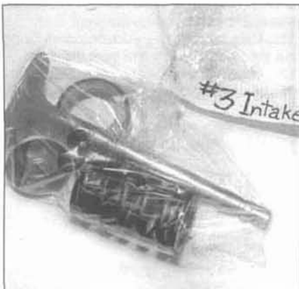
18.2 A small plastic bag, with an appropriate label, can be used to store the valve train components so they can be kept together and reinstalled in the original position
