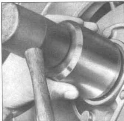
6.8 Using a socket with an outside diameter slightly smaller than the outside diameter of the seal, drive it into place
