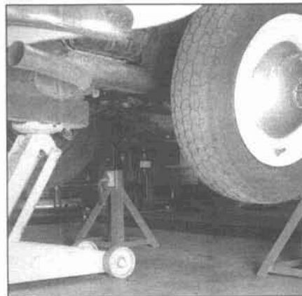
12.21 Position the jack under the center of the engine
