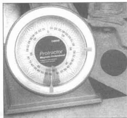
13.20 Lift the spring plate slightly to remove any freeplay, place the protractor (angle finder) on top of the spring plate and record the indicated angle
