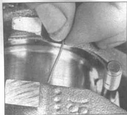
31.3 Lay the Plastigage strips on each rod bearing journal, parallel to the crankshaft centerline
