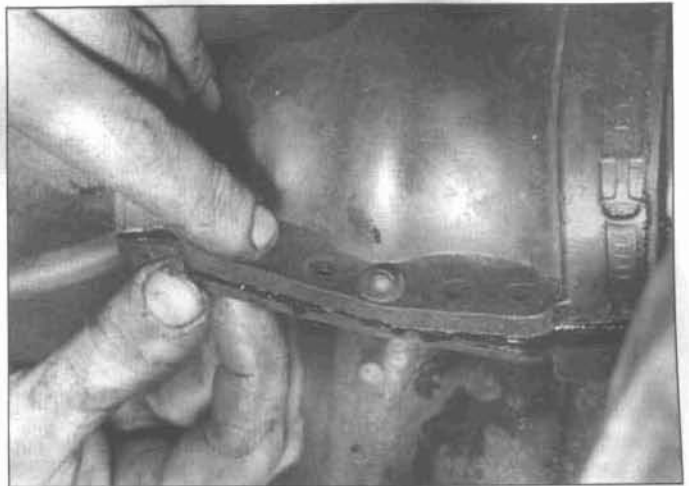
9.6a Pinch the mating surfaces along the seam together, then install the screws, washers and nuts - don't overtighten them or the boot will leak
