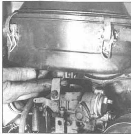
7.7a Lift the air cleaner assembly straight up
