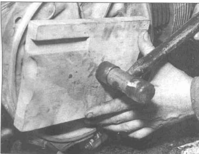
37.4b . . . and press it into place with a hammer and a block of wood . . .
