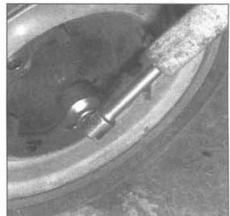
2.3l Break the rear axle nut loose with a breaker bar
