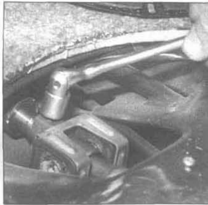
3.18b To disconnect the later type shift rod coupling, remove this bolt and the self-tapping screw on the side, then knock out the spring pin with a hammer and punch
