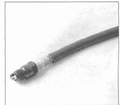
25.10 A length of 3/8-inch ID rubber hose will save time and prevent damaged threads when installing the spark plugs
