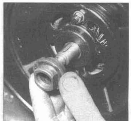
12.7b . . . and slide the hub off
