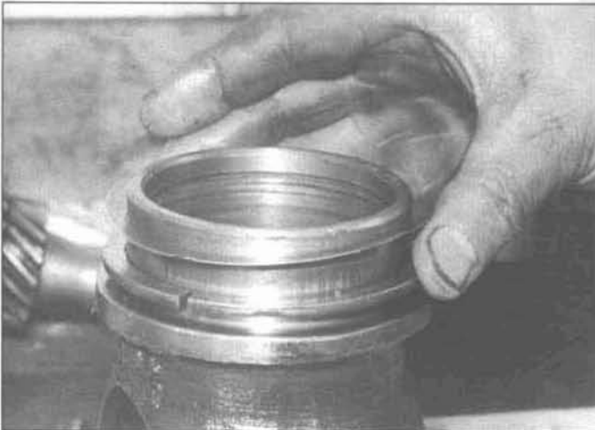
9.95 Install the differential shims and hold them in position with a dab of grease
