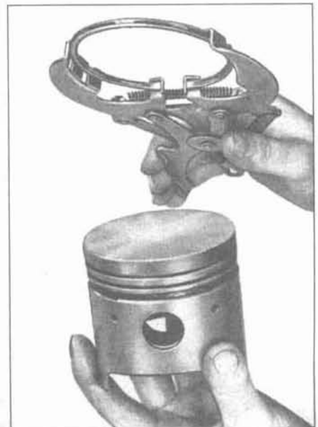
22.3 Expand the rings with a special tool and slip them over the piston
