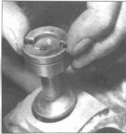
8.11a Apply engine oil to the distributor driveshaft and install it with the slot approximately perpendicular to the crankcase centerline seam and the smaller segment toward the crankshaft pulley
