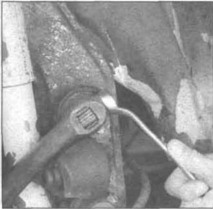
7.5a To detach a torsion arm from the torsion bar, loosen the locknut on the set screw on the inner end of the arm . . .
