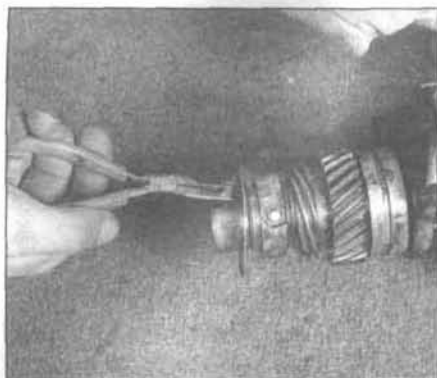
23.11a Carefully remove the Woodruff key
