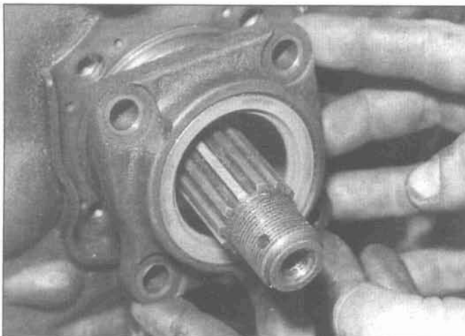
8.12 Be careful when you install the bearing cover, or you could easily damage the seal lip on the axle shaft splines
