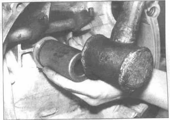
4.6 Use a large socket with an outside diameter slightly smaller than the outside diameter of the seal to drive the seal into place
