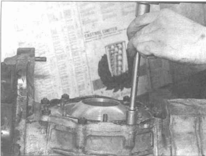
9.98c Install the cover nuts only after you have driven it into place
