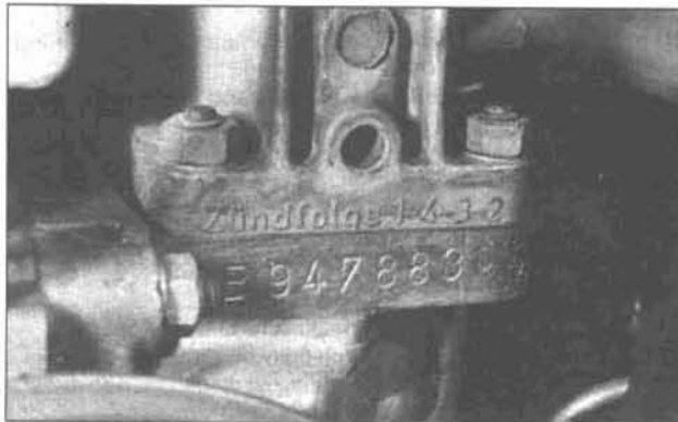
The engine identification number is stamped on the engine case, just below the generator pedestal
