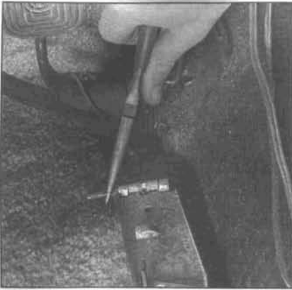
3.3 To remove the accelerator pedal, pry the pedal return spring out of the way and pull out the pedal pivot pin
