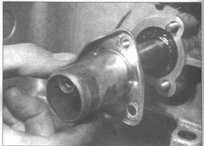
9.87d On later units, install the sleeve over the input shaft extension
