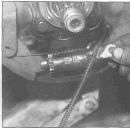
2.3q Pull the parking brake cable guide and cable through the backing plate and detach the cable from the guide
