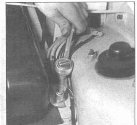
5.10 Remove the four mounting bolts and lift the fuel tank from the vehicle
