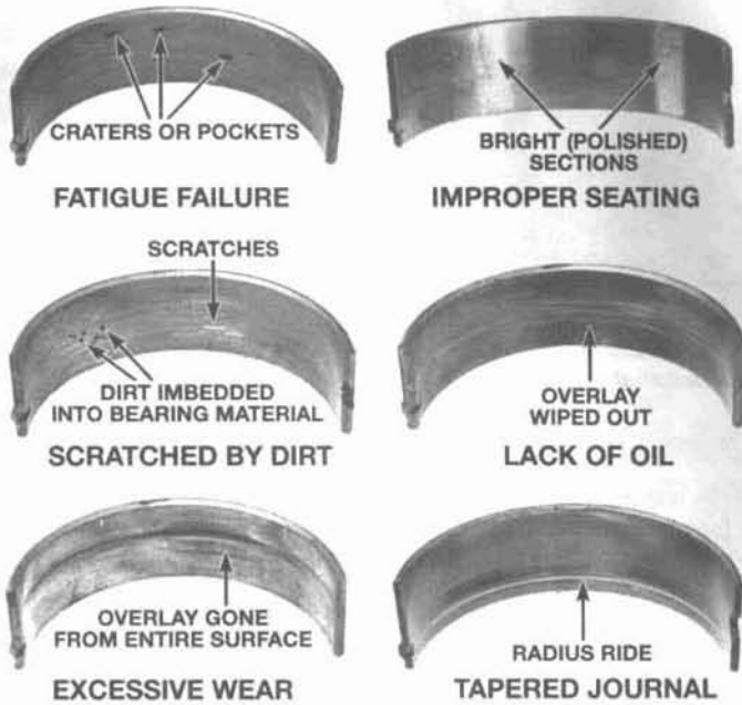
29.1 Typical bearing failures
