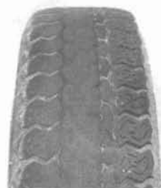
INCORRECT TOE-IN OR EXTREME CAMBER
