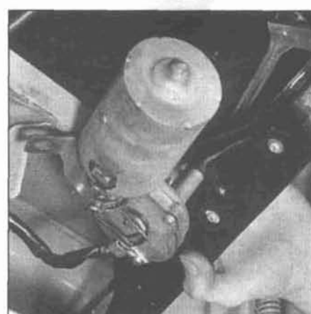
15.21 Remove the motor (1973 or later type shown, others similar)
