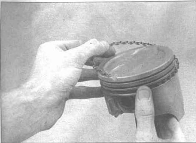
33.9 Installing the spacer/expander in the oil control ring groove
