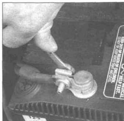
6.6b Removing the cable from a battery post with a wrench - sometimes a special battery pliers is required for this procedure if corrosion has caused the deterioration of the nut hex (always remove the ground cable first and hook it up last!)
