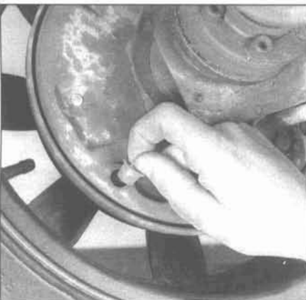
15.9 On models with four lug wheels, remove the inspection plugs to check the brake shoes
