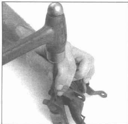
3.8 Drive out the pin which secures the clutch pedal to the shaft
