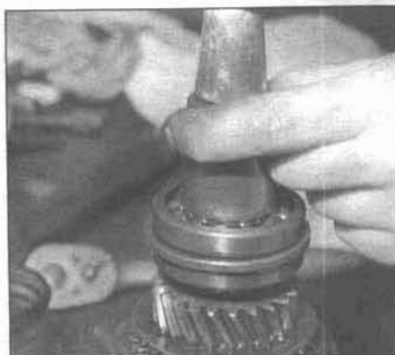
7.49b . . . and drive it on until it's fully seated against the shims
