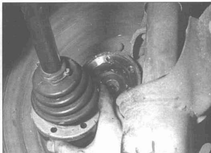
11.3 To remove a driveaxle, simply unbolt the inner and outer CV joints from the final drive flange and the stub axle, respectively (outer CV joint shown)
