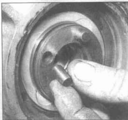
38.2 Insert the dowels, if they were removed
