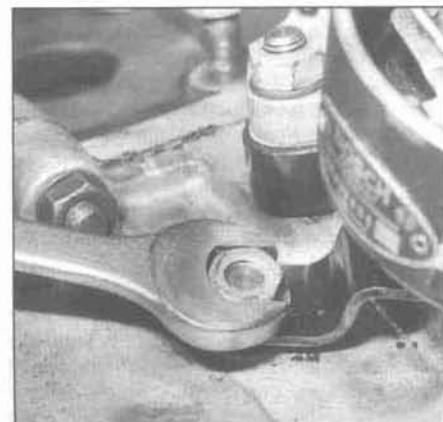
8.5 Remove the distributor hold-down nut
