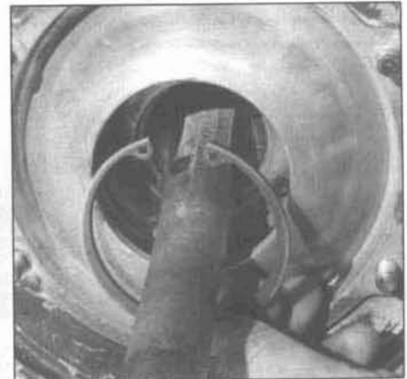
10.22c . . . and install the lock-ring (snap-ring) - make sure it seats properly into its groove in the axle bore of the differential
