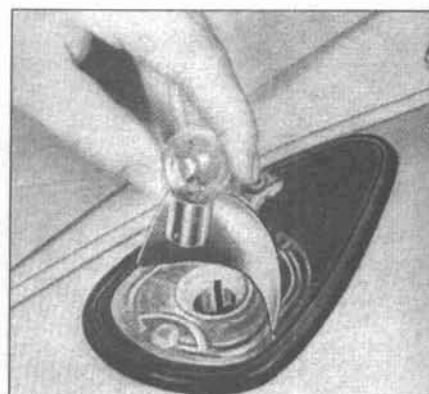
11.1c . . . press the bulb down lightly, turn it counterclockwise and remove it
