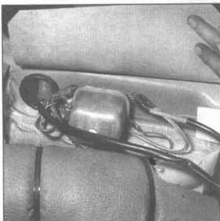
11.2a On 1967 through late 1974 model Beetles, the voltage regulator is mounted under the rear seat on the driver's side
