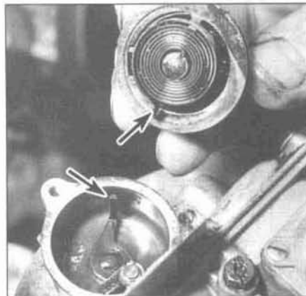
10.28a Install the bimetallic spring so the hook engages the lever (arrows)
