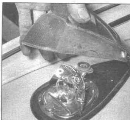
11.1b . . . remove the housing . . .
