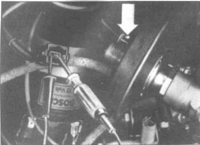
5.7 Unplug the connector (arrow) and check for idle roughness, then probe the terminals with a test light
