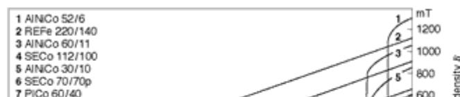
Demagnetization curves for various permanent-magnet materials
