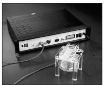
Figure 2.TC-202A Temperature Controller
