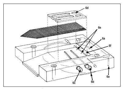
Figure 6. Placement of the Thermistor Probe
