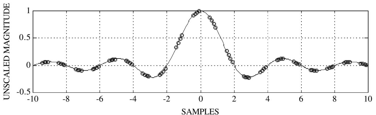
**Figure 4: Possible Downsampling Filter from 96 kHz to 44.1 kHz**
