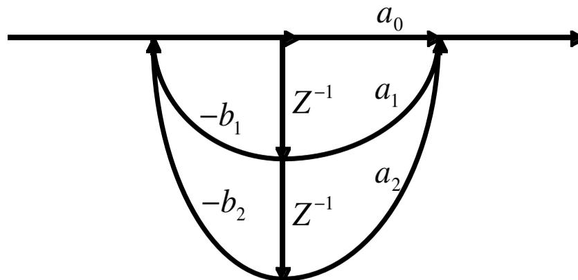
**Figure 1: One form of a second-order digital filter**
