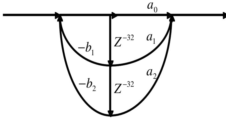
**Figure 8: Possible second-order digital filter for DSD**
