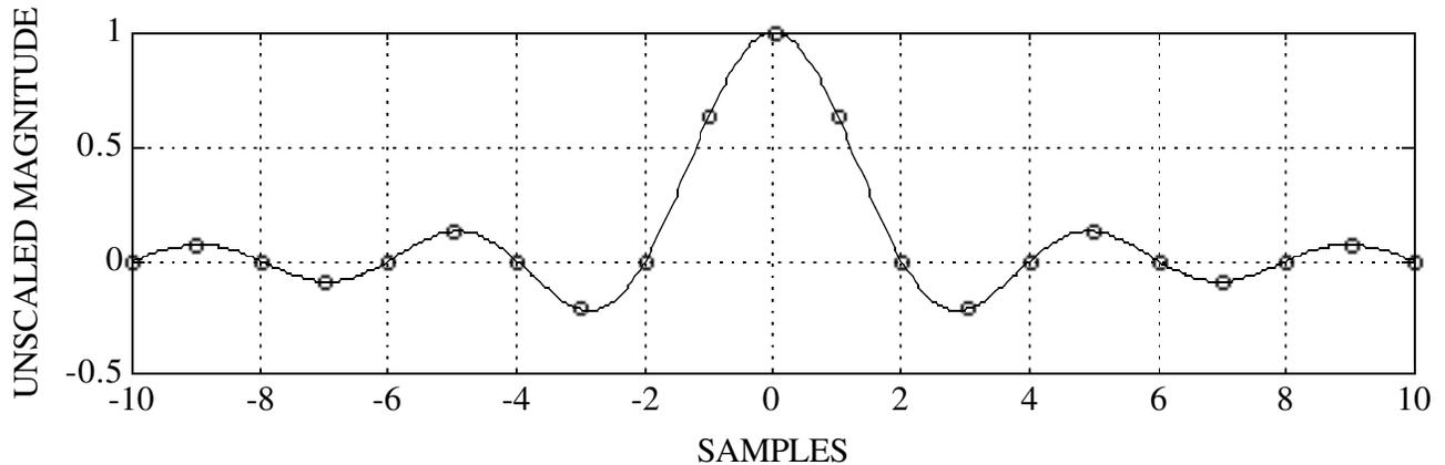
**Figure 3: Possible Downsampling Filter from 96 kHz to 48 kHz**
