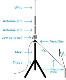
Try placing the coil on top of the feedpoint. Thread two dipole arms vertically and a fully extended whip on top. Tune single sloping and elevated radial for resonance.
