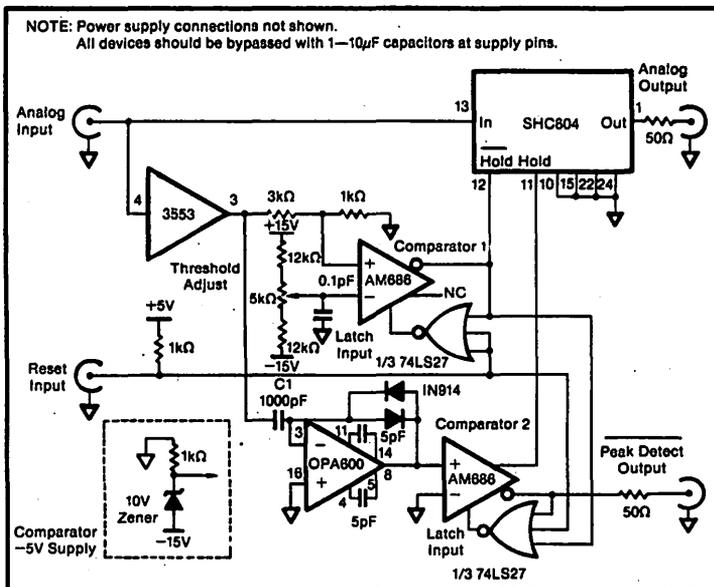
FIGURE 1. Schematic.
