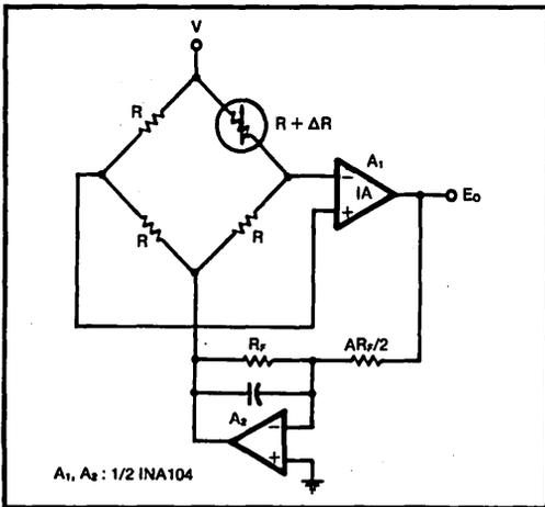
FIGURE 3. To cancel bridge nonlinearity, utilize feedback modulation of the bridge bias voltage.
