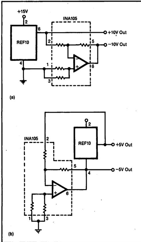
FIGURE 1. To develop precise reference-voltage generators, simply configure the INA105 as a unity-gain inverting amplifier. In the  $\pm 10\text{V}$  reference circuit (a), the INA105's low gain- and offset-temperature drifts add only about  $2\text{ppm}/^\circ\text{C}$  to the reference temperature drift. In the  $\pm 5\text{V}$  reference circuit (b), you can operate the REF10 from supply voltages that are lower than the zener voltage.
