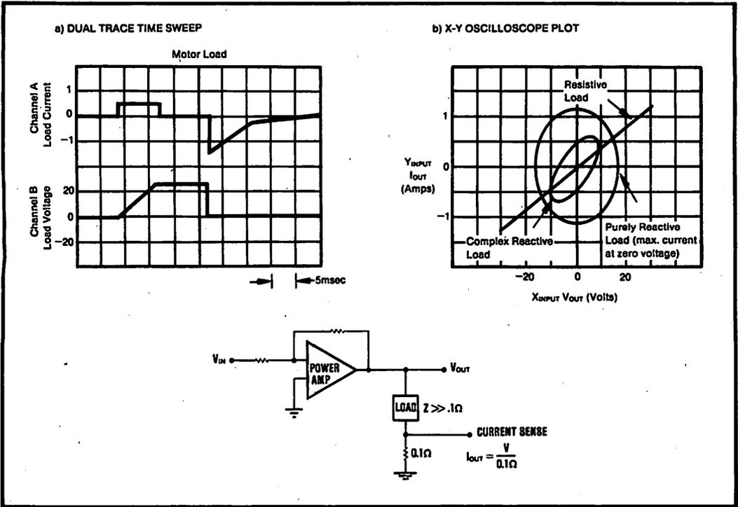
FIGURE 12. Many measurement schemes can be helpful in determining conditions of unusual loads. Setup "a" is useful in analyzing the duration of worst case conditions with motor loads. A storage oscilloscope is used to capture
