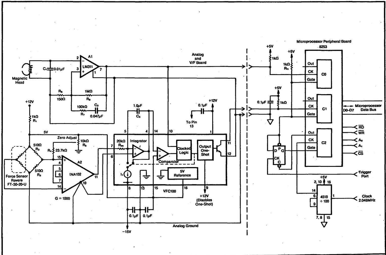
FIGURE 3. The output from the comparator, which reads the rotational speed of the wheel, serves as the clock input to the V/F converter. The strain gauge output, fed through an instrumentation amplifier, is then applied to the V/F converter. Counter outputs are applied to a microprocessor to produce—under program control—the power, torque, and rpm developed.
