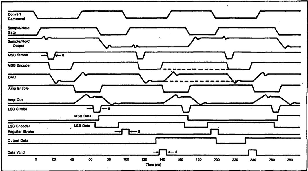
FIGURE 4. Timing Diagram of 12-Bit 10MHz ADC600.
