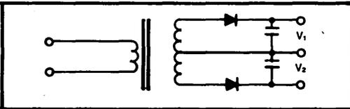
FIGURE 11. Dual-Output Converter.
