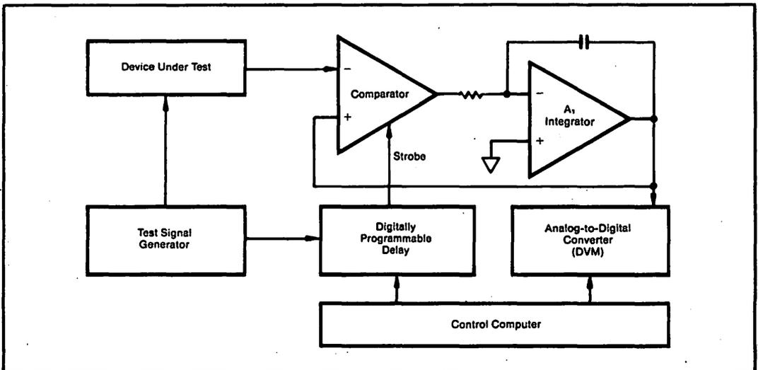
FIGURE 1. Block Diagram of the Sampling Waveform Digitizer.
