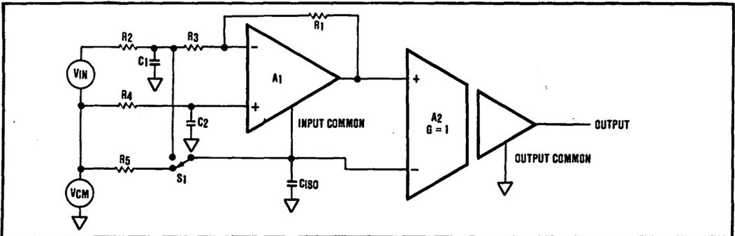
FIGURE 9. Isolation Amplifier Model For Analyzing Isolation-Mode Rejection.
