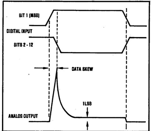
FIGURE 1. Response of Digital-to-Analog Converter in Presence of Digital Data Skew.
