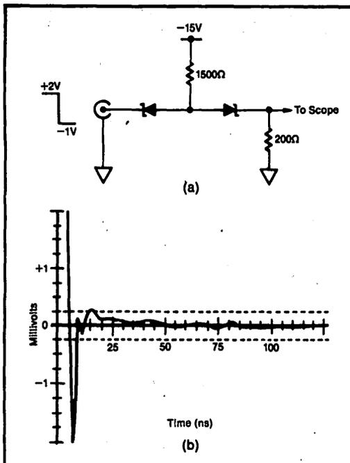
FIGURE 9. Schottky Diode Test Circuit and Resultant Plot.
