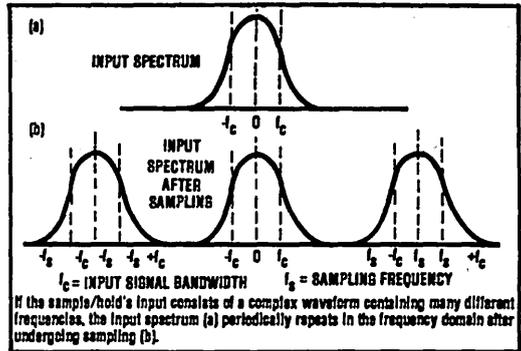
If the sample/hold's input consists of a complex waveform containing many different frequencies, the input spectrum (a) periodically repeats in the frequency domain after undergoing sampling (b).
