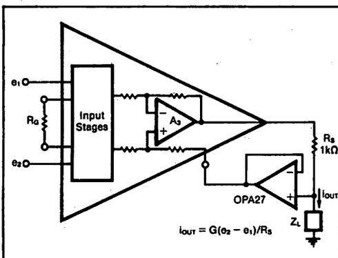
FIGURE 6. Current output is attained by reconfiguring the difference amplifier when the needed circuit points are supplied (a), or by bootstrapping the amplifier from the load when they are not (b).
