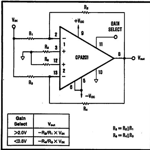
FIGURE 7. Selectable-Gain Amplifier.
