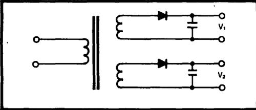
FIGURE 10. Dual-Channel Converter.
