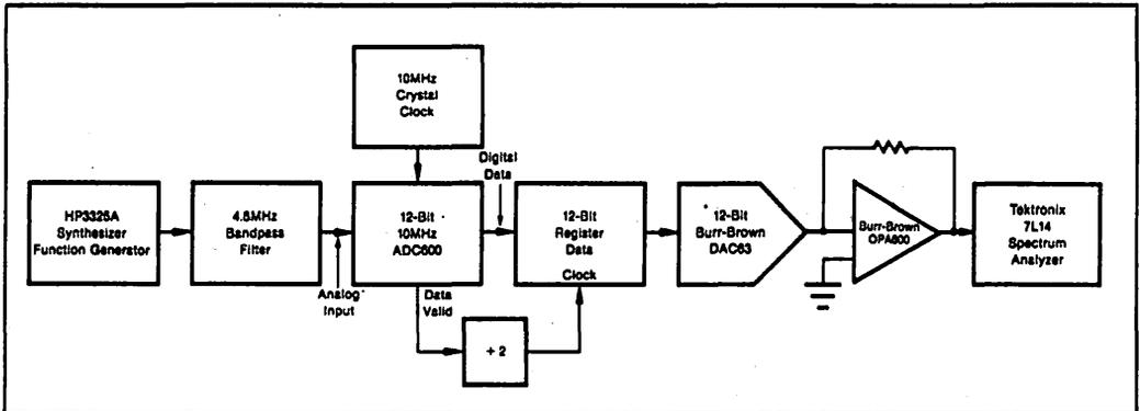
FIGURE 13. Block Diagram of Spectrum Analyzer Test.
