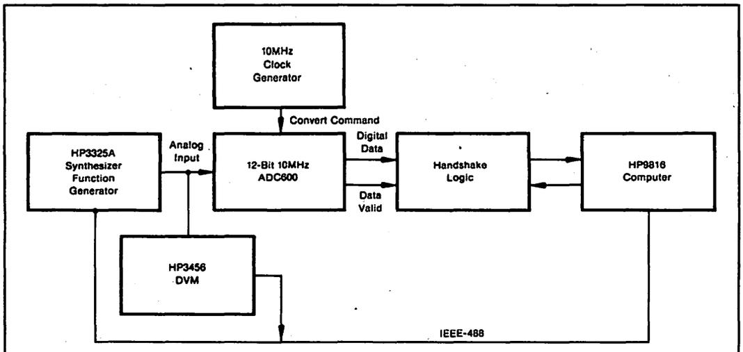
FIGURE 11. Block Diagram of Histogram Test.
