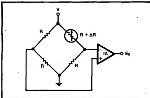
FIGURE 1. Undesirable nonlinearity and drift sensitivity result when you use an instrumentation amplifier for bridge monitoring.
