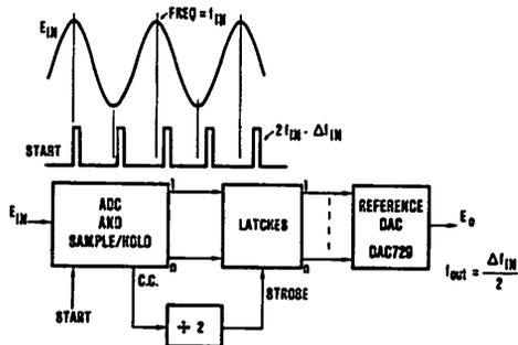
FIGURE 9. Test Circuit for a High-Speed ADC.
