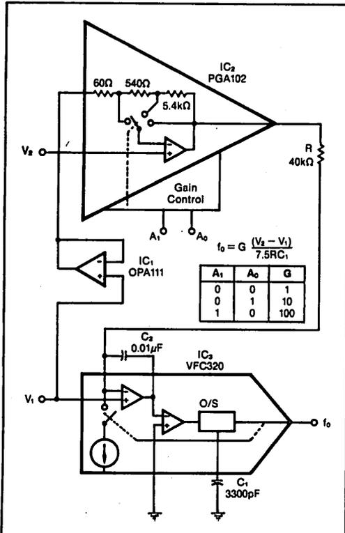
FIGURE 8 .By adding op amp  $IC_1$  to the circuit in Figure 7, you create an instrumentation-amplifier input without affecting either the circuit's frequency range or its digital-gain-control capabilities.
