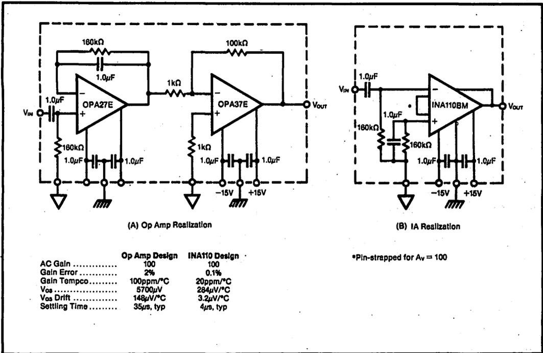
FIGURE 5. AC-Coupled Inverting Amplifier (-3dB = 1Hz).
