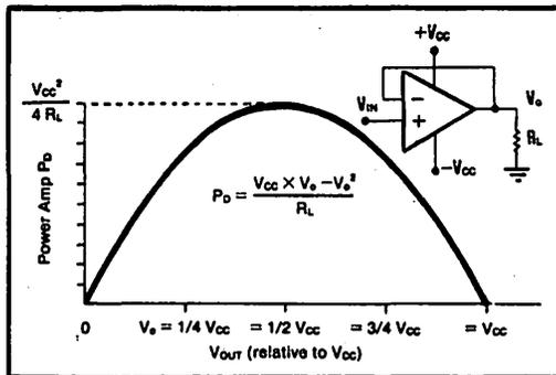
FIGURE 6. The power dissipation for a simple resistive load and DC input signal is at a maximum when the output voltage is  $V_P/2$ . Despite the larger currents at higher output voltages, the dissipation is actually lower. It approaches zero as the  $V_{CC}$  nears zero at maximum output voltage.
