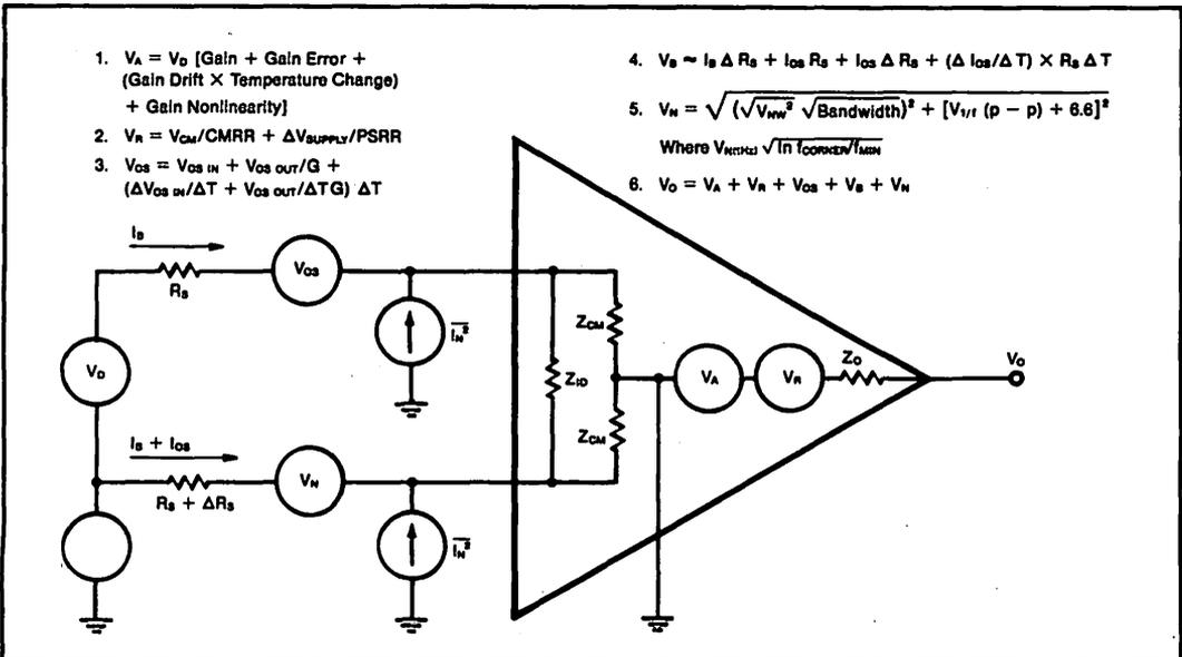
FIGURE 6. You can best compare instrumentation amplifier performance by analyzing all possible error sources. Note that gain and drift errors are referred to the input.  $V_{NW}$  is the white-noise magnitude in the white-noise region; the 6.6 divisor in Eq 5 is a crest factor that converts a 0.1%-probable peak value to rms.
