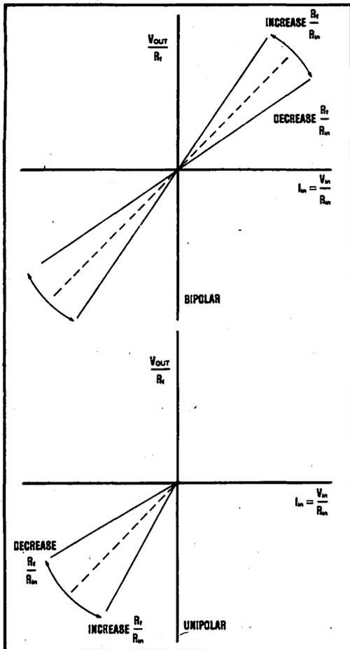
FIGURE 8. ADJUSTING THE GAIN. Changing the ratio  $R_f/R_{in}$  will change the gain by rotating the transfer function about the point where  $I_{in} = 0$ . This will be true for both the unipolar and bipolar cases.  $I_{OS}$  is zero in these examples.
