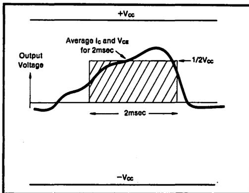
FIGURE 7. A pulsed waveform can be evaluated for safety by a graphical approximation with a rectangular pulse at the worst-case instantaneous point. The duration and conditions are then compared to the pulsed SOA data. Duty cycles greater than approximately 10% should be given plenty of guard band to allow for recovery from any localized heating during the pulse.
