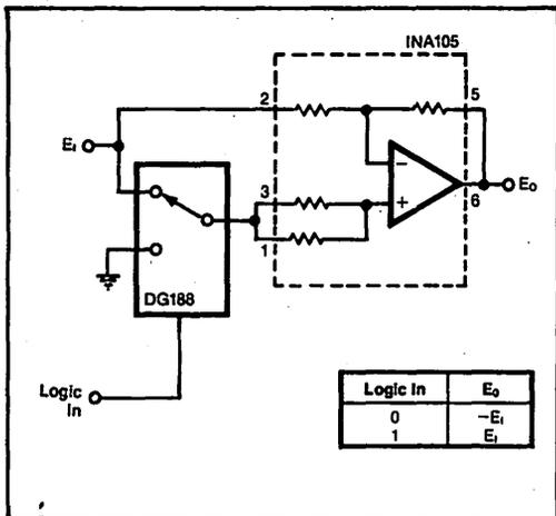
FIGURE 9. To control analog circuits with digital signals, you can configure this unity-gain buffer as an amplifier with a digitally controlled gain of  $\pm 1$ . In this figure, the DG188 analog switch acts under logic control to connect the INA105's noninverting input to either the input signal or ground.
