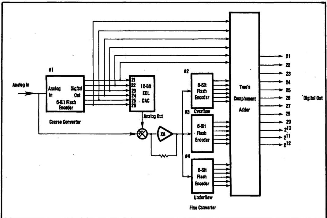
FIGURE 10. Block Diagram of 250nsec Analog-to-Digital Converter.
