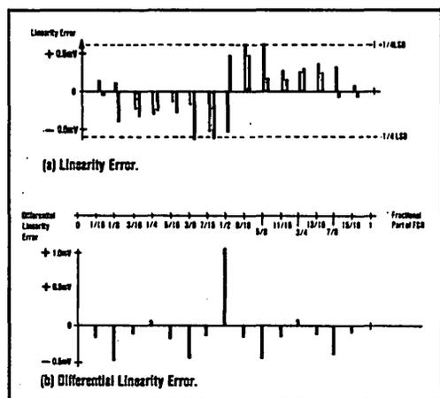
FIGURE 2. DAC85 Errors at 15 Evenly Spaced Carries.
