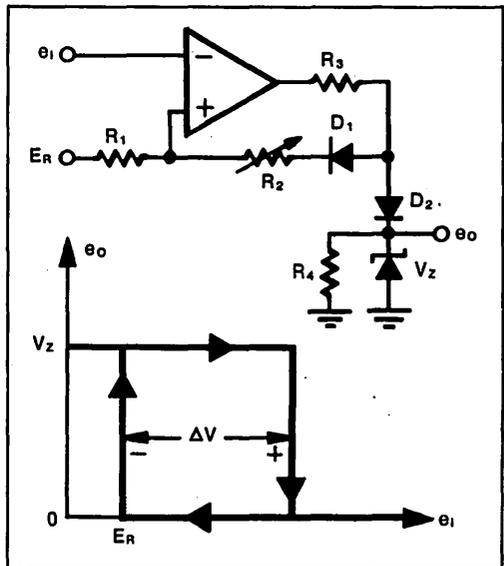
**CONTROLLABLE HYSTERESIS.** Positive feedback circuit for analog op-amp comparator does not shift the initial reference trip point while introducing hysteresis in the second trip point. The voltage difference,  $\Delta V$ , between the trip points can be adjusted by varying resistor  $R_2$ . When the output voltage is taken from the zener diode, as shown, it switches between zero and  $V_Z$ , the zener voltage.
