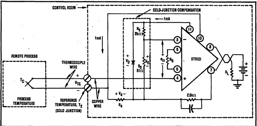
FIGURE 4. The thermocouple, a popular device for sensing temperature, needs cold-junction compensation to generate an absolute output. A reference diode,  $V_D$ , tracks the ambient temperature to perform the compensation.
