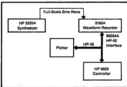
FIGURE 6. Setup for histogram test.
