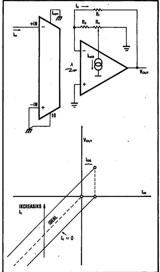
FIGURE 5.  $I_{OS}$  ADJUSTMENT FROM THE OUTPUT SIDE. Connecting a negative correction current ( $I_c$ ) to the summing node of the output amplifier causes the transfer curve to shift upwards by the amount of  $I_c$ . This causes the output to shift toward zero. Again, a current divider is used to derive the correction current from the internal references. By combining the methods of Figures 4 and 5, a correction current can be generated that will cancel either polarity of  $I_{OS}$ .
