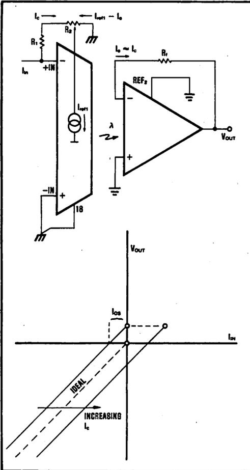
FIGURE 4.  $I_{OS}$  ADJUSTMENT FROM THE INPUT SIDE. If  $I_{OS}$  were negative, the ideal transfer curve would be shifted to the left, as shown above. This would cause a positive output voltage when there was no input current. Connecting a negative correction current,  $I_c$ , to the summing node of the first op amp causes the transfer curve to shift to the right. Thus, the effect of  $I_{OS}$  can be trimmed out.
