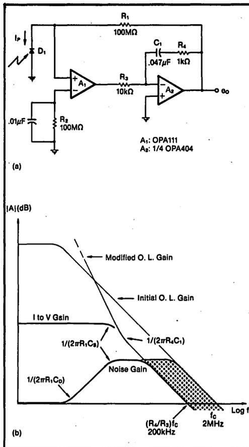
FIGURE 5. Noise reduction results with (a) a composite amplifier that (b) restricts noise bandwidth without reducing that of the signal.
