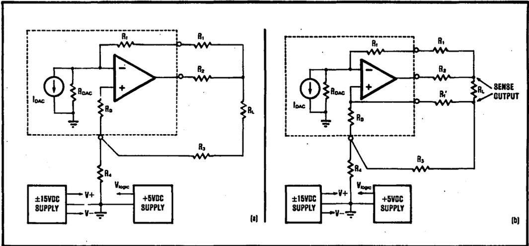
FIGURE 5. These connection diagrams show how to reduce the effects of wiring and socket resistance for a typical DAC (a) and a high accuracy DAC (b). Resistors  $R_1$ ,  $R_2$ ,  $R_3$ , and  $R_4$  represent wiring and contact resistance.
