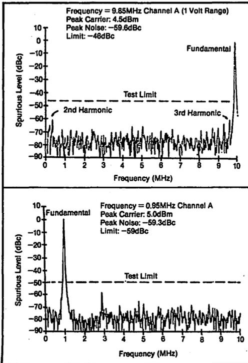
FIGURE 15. DFT plots for the 5180A with input frequencies of 9.85MHz (top) and 0.95MHz (bottom). The low harmonic distortion indicates very low integral nonlinearity.
