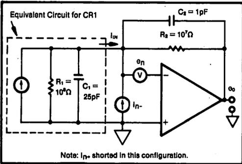
FIGURE 4. Noise Model of Photo Diode Application.
