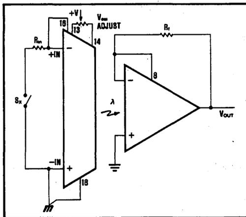
FIGURE 10. PREFERRED METHOD FOR VOLTAGE OFFSET TRIM. In those rare applications where offset voltage is significant, it is best to adjust the input offset voltage,  $V_{OS1}$ , as shown above.  $V_{OS1}$  and its drift appear at the output multiplied by the factor  $R_f/R_{in}$ .  $V_{OS1}$  will usually not be gained up, and thus will not need adjustment. Adjust  $V_{OS1}$  until opening up and closing  $S_1$  causes no shift in the output voltage.
