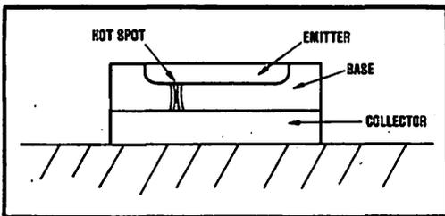
FIGURE 3. At high  $V_{CE}$  and  $I_C$ , localized hot spots may cause a localized burn-out producing a collector-emitter short—the ultimate result of secondary breakdown.
