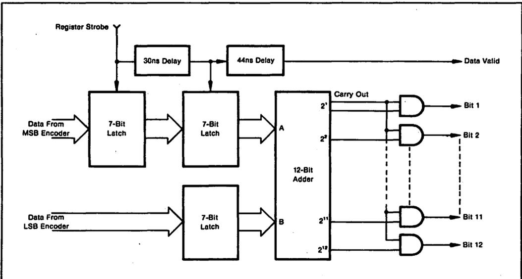
FIGURE 9. Block Diagram of Digital Error Corrector.
