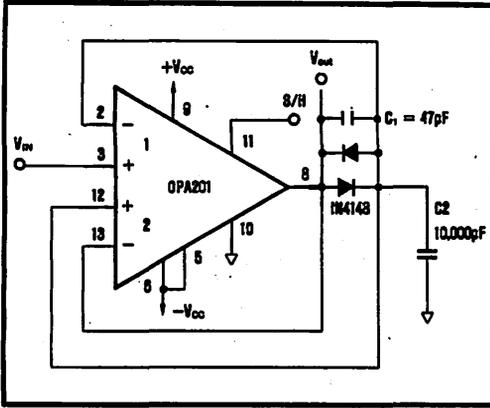
FIGURE 10. Low Power Sample/Hold Amplifier.
