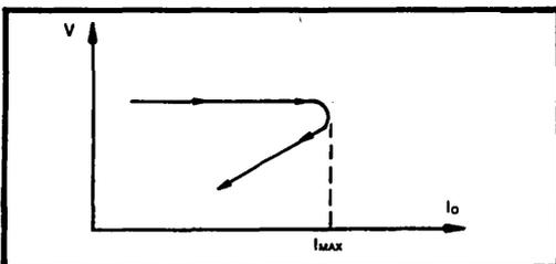
FIGURE 12. Foldback Circuit.
