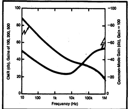
FIGURE 3. You can improve the common-mode rejection for worst-case mismatches of time constants  $R_1C_1$  and  $R_2C_2$  in the Figure 2 circuit by adding a small trimming resistor in series with  $R_1$  and  $R_2$ .
