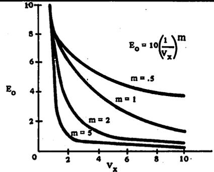
FIGURE 6a. Exponentiator Transfer Characteristics for  $(\frac{1}{V_x})^m$ .
