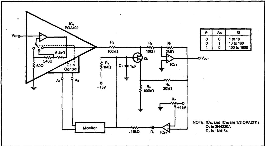
FIGURE 3. This automatic gain-control circuit maintains  $V_{OUT}$  at a set peak level for input signals having an 1800:1 dynamic range. The monitor circuit is equivalent to a 2-bit A/D converter that sets the PGA's prescale gain.
