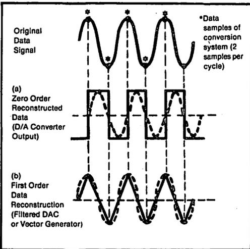
FIGURE 3. Reconstruction of Sampled Data Where  $f_s = 2 f_{max}$ .
