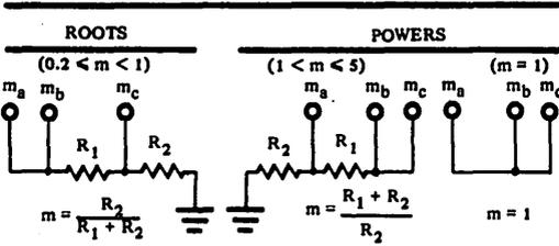
FIGURE 2. Exponent Selection for Multifunction Circuit. Resistors  $R_1$  and  $R_2$  from a voltage divider. For  $m$  less than one, the log ratio output is simply attenuated by  $R_1$  and  $R_2$ . For  $m$  greater than one,  $R_1$  and  $R_2$  determine the gain of the log ratio amp.
