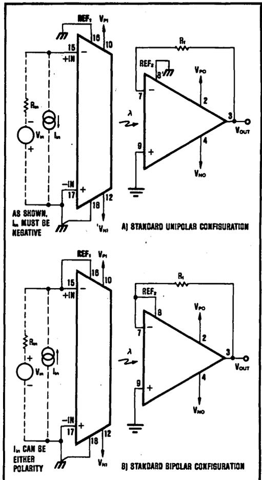
**FIGURE 3. STANDARD CONFIGURATIONS.** Most applications of the ISO100 will make use of these configurations, with slight variations. (A) shows the configuration for unipolar operation, which functions for negative inputs only. (B) shows how to use the internal references to provide bipolar operation. The circuits show all necessary connections and indicate the package pin numbers. Note that power supply connections ( $V_P$  and  $V_N$ ) to the input and output stages must be "isolated."
