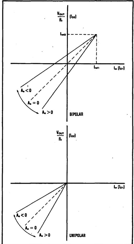
FIGURE 7. EFFECT OF GAIN ERROR ( $A_e$ ).  $A_e$  will cause an error in the slope of the transfer function, rotating the line about a point determined by the quiescent current in D1 and D2. Unipolar, this point is near the origin. In the bipolar mode, the internal references cause this point to shift to the right and up as shown above. In either case, the change in slope is the same.
