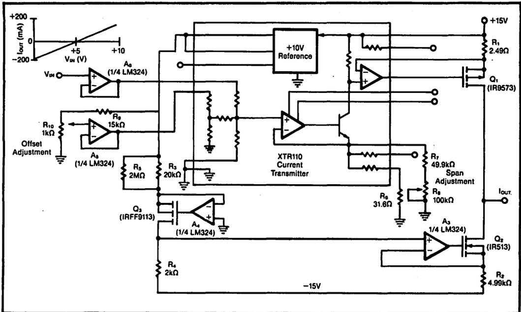
FIGURE 5. Alterations to the support circuitry to the current transmitter allow it to accommodate actuators that require a bipolar current. Resistors  $R_1$  and  $R_2$  feature low temperature coefficients and dissipate just 0.2W continuously;  $R_4$  and  $R_{10}$ , two 10-turn potentiometers, afford great sensitivity.
