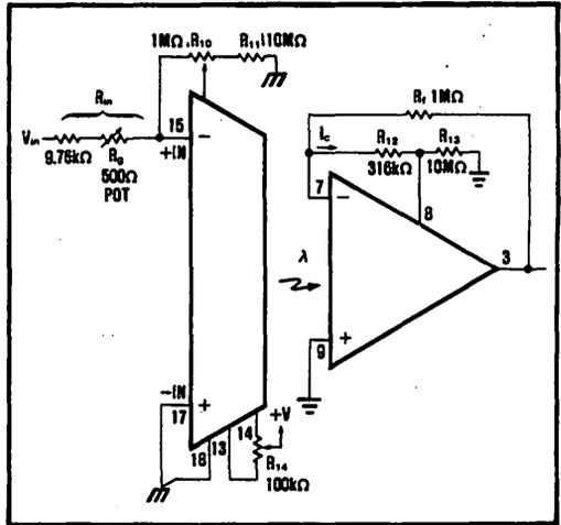
FIGURE 12. ADJUSTING THE BIPOLAR ERRORS (EXAMPLE 4). Each of the errors are adjusted in turn. With  $V_{in} = \text{"open"}$ ,  $I_{Os}$  is trimmed by adjusting  $R_{10}$  to make the output zero.  $R_8$  is then adjusted to trim the gain error. The effects of offset voltage are removed by adjusting  $R_{14}$ .
