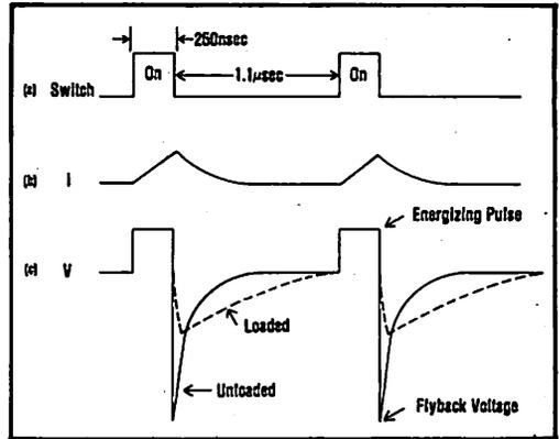
FIGURE 2. Flyback modulation. The pulsed supply voltage is applied to transformer winding (a). As a result of voltage  $V$  across winding, current  $i$  increases as in (b) until switch opens, producing flyback shown in (c). Rectified positive-going pulses provide power to energize input op amp  $A_1$  which controls flyback modulator.
