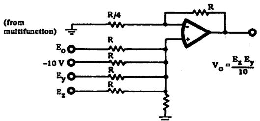
FIGURE 11. Additional Circuitry of Obtain Four-Quadrant Multiplier.
