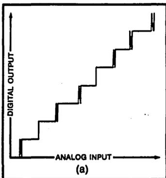
FIGURE 9. Averaging five consecutive conversions of the ADC76KG cleans up some the transition noise (a). The effect of averaging 10 conversion (b) is and even cleaner transfer function, but only at the expense of a longer effective conversion time ( $150\mu\text{s}$ ).
