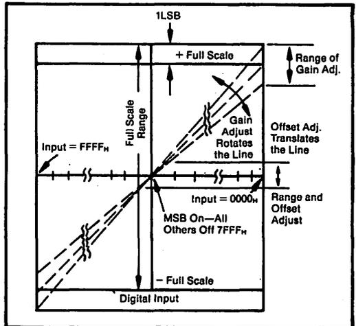
FIGURE 2b. DAC Gain Adjust Rotation Using REF ADJ Pin.
