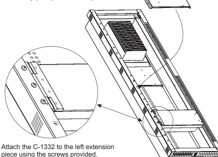
Note: There are 6 possible locations where the C-1332 Hinged Mounting Plates can be attached to the C-1355 Extender Ring. This provides the installer with multiple mounting options. However, to maintain proper operating temperatures, no more than 4 amplifiers should be installed at one time.
