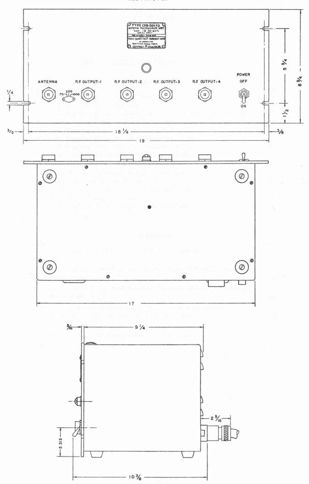
Figure 13—Type CKB-50172. Antenna Multicoupler Unit, Outline and Mounting Dimensions
