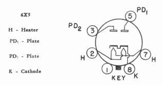
Alphabetical subscripts D, P, T, and HX indicate, respectively, diode unit, pentode unit, triode unit, and hexode unit in multi-unit types.
