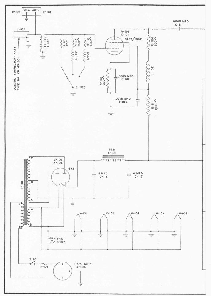
Figure 14—Type CKB-50172 Antenna Multicoup
