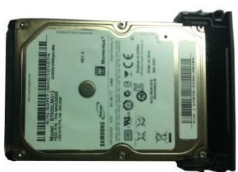
② Make sure the HDD metal surface is facing up and then put the HDD into the bracket horizontally. After the HDD is in
