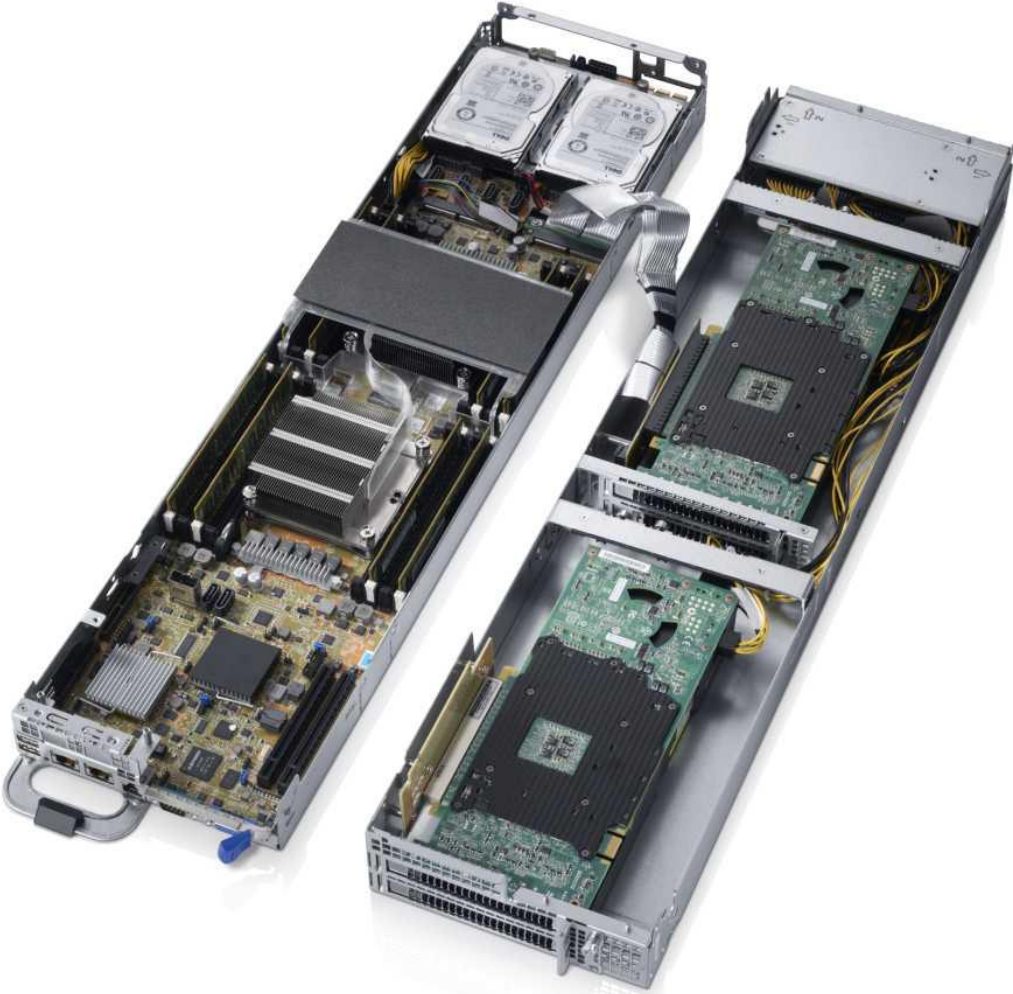
Figure 12. PowerEdge C8220X sled interior view
