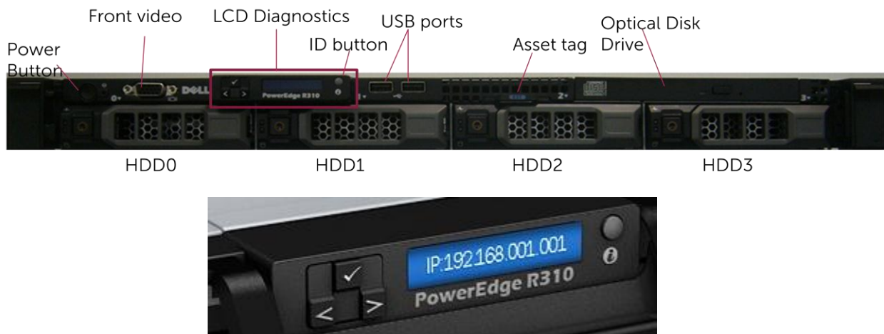
Figure 3. Front View Hot-swap HDD Configuration with LCD Panel
