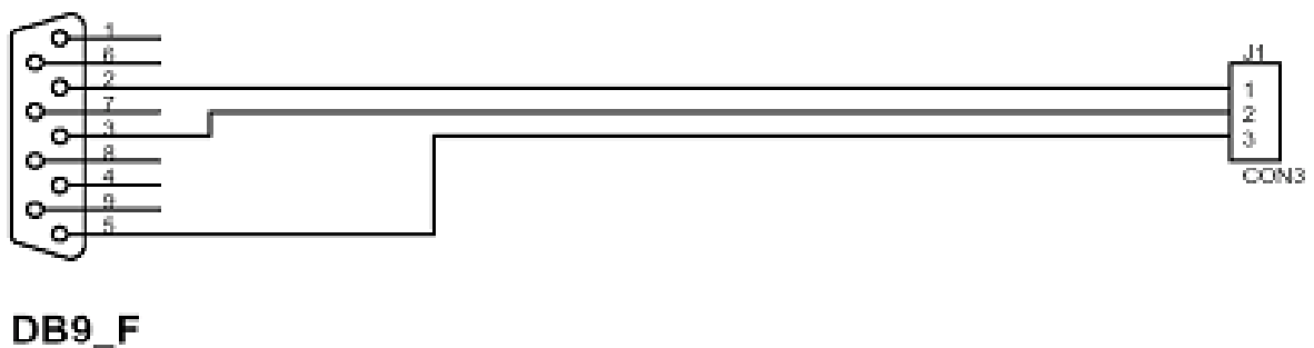
Figure 60: MVX-A16 serial cable (CAB-MVX-48Z)
