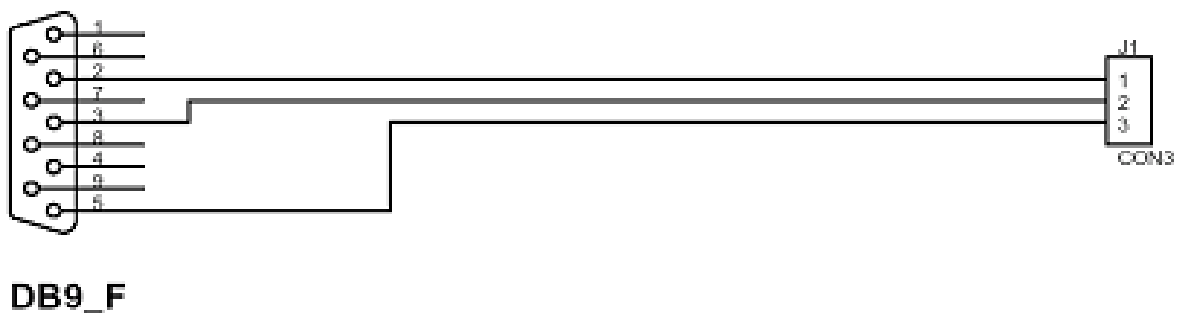
Figure 55: MVX-A16 serial cable (CAB-MVX-48Z)
