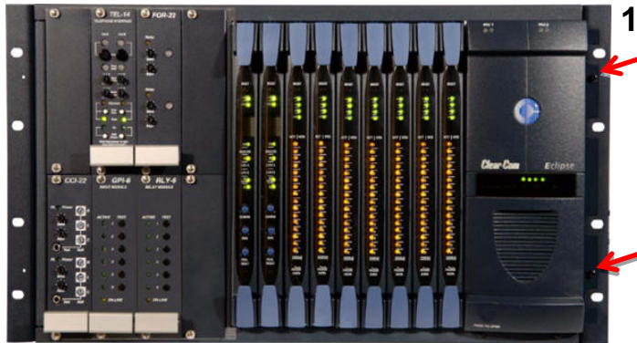
Figure 2: Screws securing the Eclipse door (and hinge) unit
