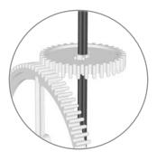
Another type of gear, known as a **rack and pinion**, comprises a small spur gear (a pinion) that meshes with a toothed bar (a rack) rather than another toothed wheel. This means that as the pinion is turned it pushes against the teeth of the rack making it move sideways in a straight line and produces linear motion. If the rack is moved, then the pinion can be made to rotate. The rack and pinion mechanism can be used to convert rotary to linear motion and linear to rotary motion.
