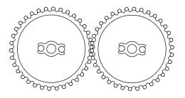
Spur gears lie in the same plane and turn in opposite directions, but only when they mesh together. Different sized spur gears turn at different speeds and with different amounts of force. Try it!
