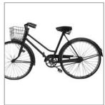
Gears can also be connected using chain links – as in a bicycle. Gears used with chains are called **sprockets**. Sprockets do not mesh with other gear wheels but with the links in the chain. When moved, they turn in the same direction. As with spur gears, different sized sprocket gears turn at different speeds and with different amounts of force. If they are the same size, they turn at the same speed and with the same force.
