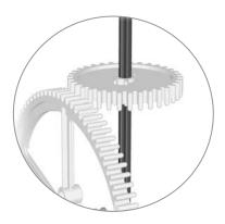
The mechanism is called a **crown gear wheel and pinion**. The pinion is simply another name for a follower gear.
