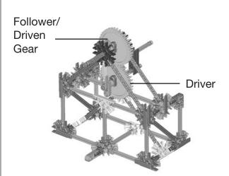
Consider a spur gear system. The first gear wheel to be turned, and the one to which the effort force is applied, is called the driver. In the K'NEX Crank fan model, the **driver** is the gear attached to the handle axle. The driver transmits turning forces to the **follower**, or **driven**, gear causing it to rotate in the opposite direction.
