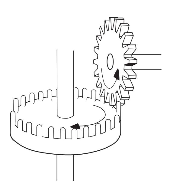
A crown gear meshes at right angles (90-degrees) to another gear and changes the direction of motion. One gear turns vertically (up and down), while the other turns horizontally (side to side).
