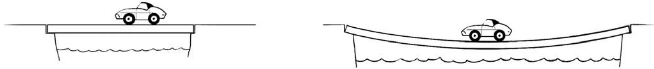
Fig. 32 - Long beams are weaker than short ones.
