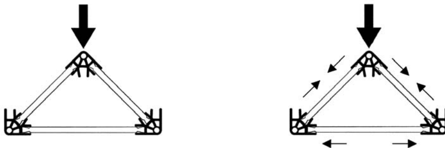
Fig. 27 - Force applied to the angle of a triangle.
