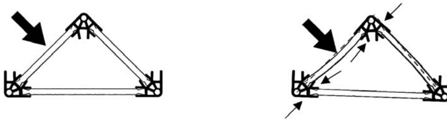
Fig. 26 - Force applied to the side of a triangle.
