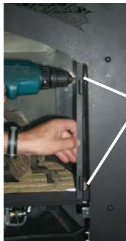
Door Bracket attaches with 2 screws on each side.
