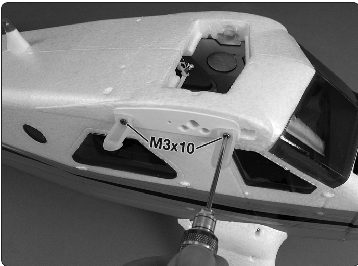
❑ 1. Fasten the wing clips to both sides of the fuselage with four M3x10 screws.
