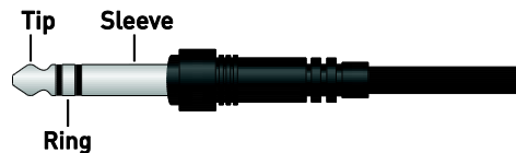
Figure 1-5: TRS Cable, AKA “Balanced” or “Stereo” Cable End
