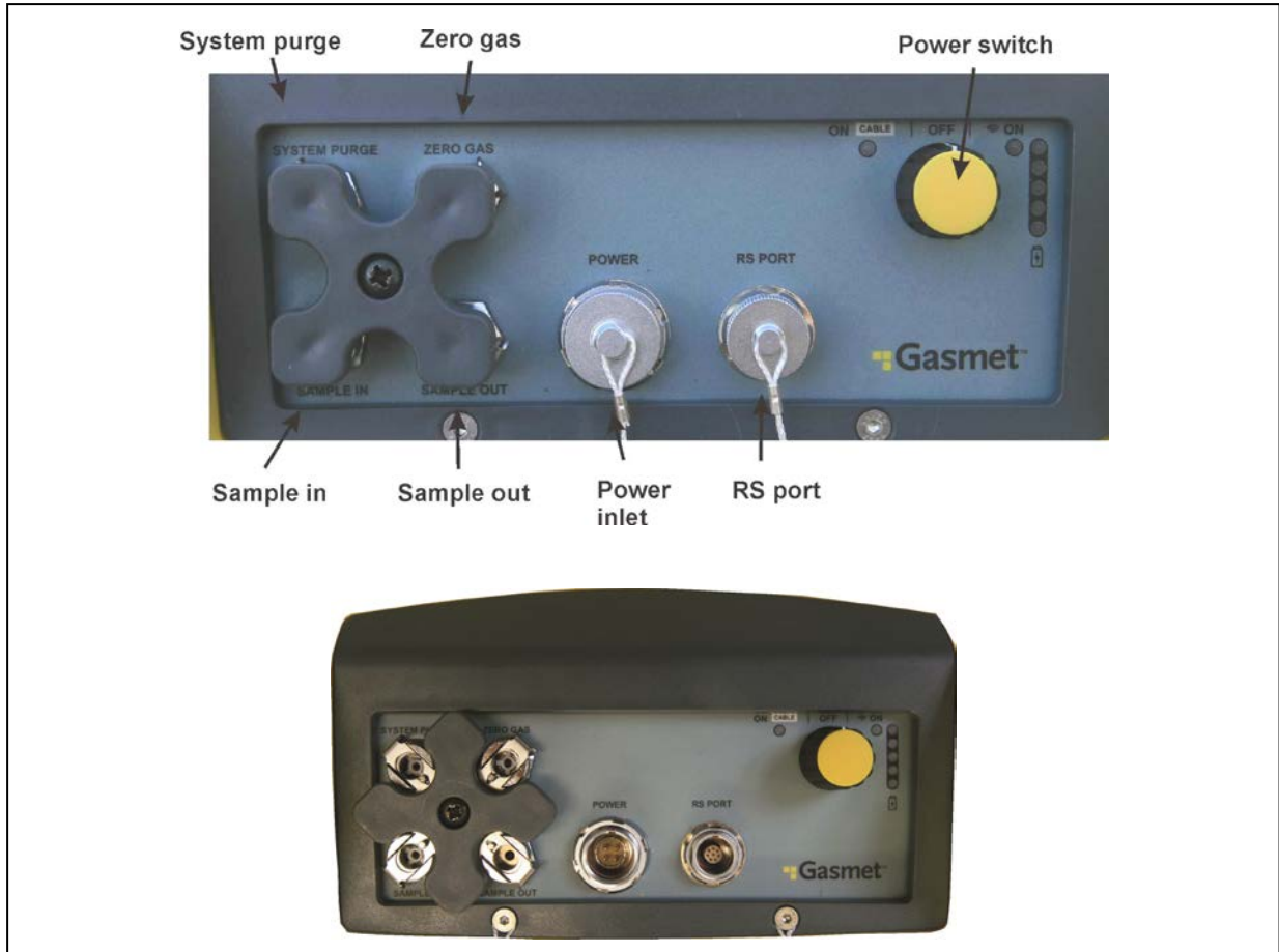
Figure 10. Front panel: sample gas fittings and connectors of the DX4040 model.
