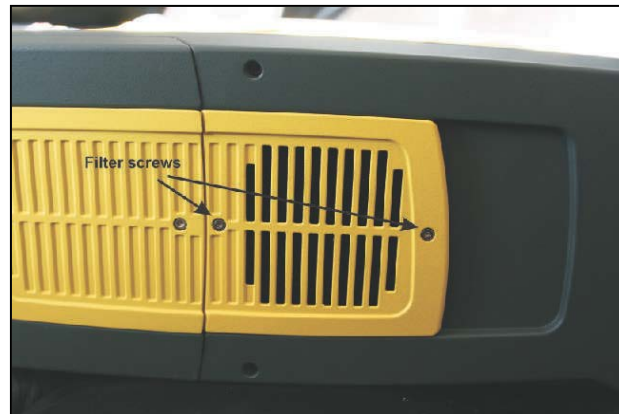
Figure 28. Dust filters cleaning.
