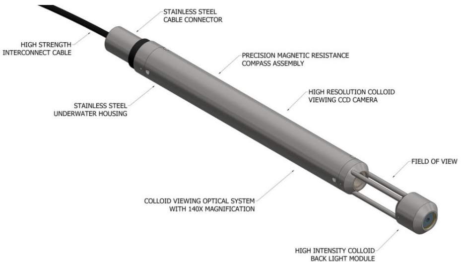
Figure 1-1: Colloidal Borescope Probe Features
