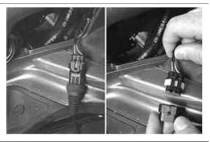
Power the diagnostic tester by connecting the terminals to the battery poles, or the specific connector to the socket inside the gloves compartment.
