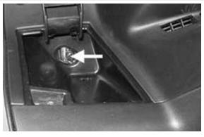
Remove the light, disconnecting the electric con-
