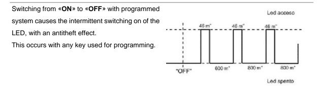
If the scooter is not used, the deterrent light stops automatically after 48 hours to prevent discharging the battery. A new 48-h cycle starts by switching from "**OFF**" to "**ON**" and "**OFF**" again.
