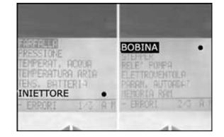
9 - The control unit has detected a failure on the line of pin 19
