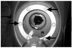
Remove the flap, the gasket, the second flap and the second gasket.
