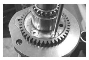
Blow with compressed air and degrease the mounting holes on both surfaces to make the new LOCTITE grip.
