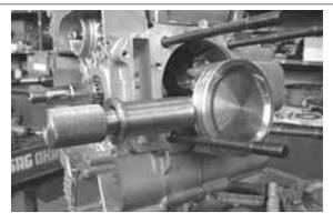
N.B. THE TOOL FOR INSTALLING THE STOP RINGS MUST BE USED MANUALLY. CAUTION USING A HAMMER MIGHT DAMAGE THE STOPS' HOUSING.
