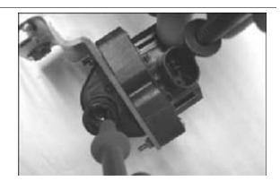
18 - The coil is conforming.
