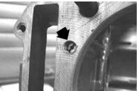
The jet clogging impairs the head lubrication and the timing mechanisms.
