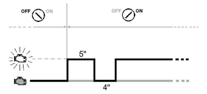
Any faults discovered in this phase are signalled via the injection light.
