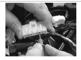
9 - Faulty led, replace the instrument panel.
