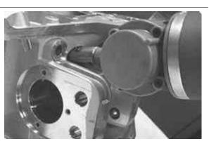
TO AVOID SCORING THE CONTACT SURFACE, DO NOT KEEP ROTATING THE VALVE WHEN NO LAPPING COMPOUND IS LEFT. CAREFULLY WASH THE CYLINDER HEAD AND THE VALVES WITH A SUITABLE PRODUCT FOR THE TYPE OF LAPPING COMPOUND BEING USED. CAUTION
