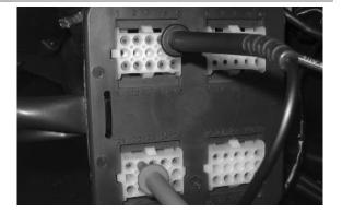
11 - If slightly higher values are detected, check the connectors.
