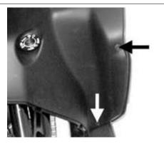
Press the shield back plate forward to allow access to the socket on the frame of the key switch.
