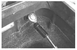
Set the switch to "**ON**" and select the diagnostic tester menu to the immobiliser function. Scroll the pages to display the control unit data.
