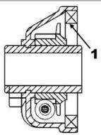
LA MRM 2 (soap-based lithium grease with Molybdenum disulphide).
