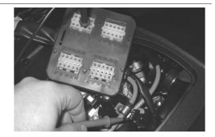
12 - Check the earth insulation of the 4 stepper lines.
