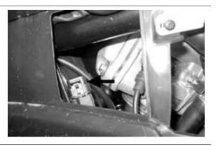
Overturn sensor In order to access the overturn sensor, remove the central union.
