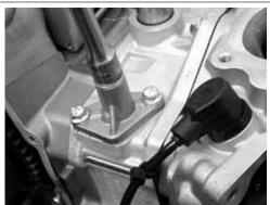
Remove the inside hexagon screw and the counterweight as shown in the figure.
