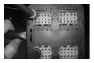
13 - Measure voltage between terminals 11 and 22. Gradually open the throttle valve and check that
