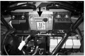
In order to access the connector, remove the windshield with the respective support and the metal plate holding the control unit ECU, decoder and saddle opener remote control.
