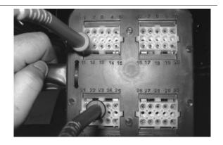
9 - Repair or replace the injection wiring
