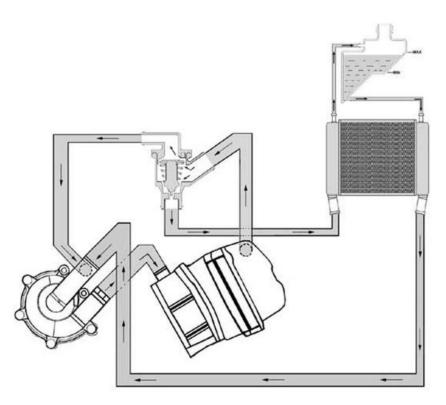
The cooling system is of the forced circulation type, with continuous venting and air pressurisation.
