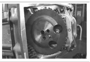
Install the engine revolution timing sensor using a new O-Ring, orientating it as shown in the figure.
