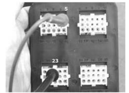
15 - Repair or replace the cable harness.16 - Connect the remote control switch and check for battery voltage between terminals 5 and 23 with the key switch in position "ON".
