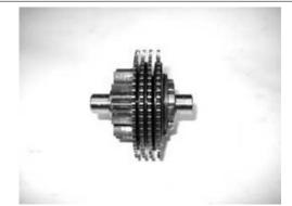
The limiter assembly cannot be overhauled. In case of irregularities on the toothed discs, replace the assembly.
