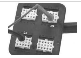
**16** - Replace the control unit. **17** - Check the presence of voltage (+ batt.) between pin 86 of the pump remote control switch and pin 23 of the control unit. Fix the wiring, if required. Check the relay coil continuity.  $85 - 86 = 100 \pm 50\Omega$
