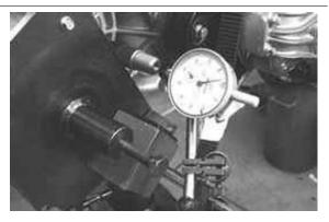
Specific tooling 020262Y Crankcase splitting strip 020335Y Magnetic support for dial gauge Characteristic Standard clearance: 0.10 - 0.50 mm Admissible increase limit after use: 0.60 mm
