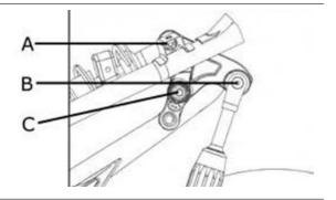
A = Connection of rear support strut to hub cover: 20-25 N-m
