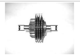
Also check the shaft diameter on the flywheel cover and on the engine crankcase.
