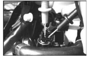
**19** - Check the earth insulation of the injector negative line. Disconnected control unit and injector connectors.
