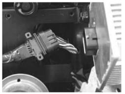
5 - Check the following conditions: PIN 1 diagnostic socket - PIN 10 control unit = continuity PIN 2 diagnostic socket - PIN 23 control unit = continuity with earth PIN 3 diagnostic socket - PIN 9 control unit = continuity 10 - 23 = insulation (>1 M $\Omega$ ) 9 - 23 = insulation (>1 M $\Omega$ ) YES go to 6 NO go to 7
