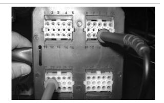
11 - If slightly higher values are detected, check the connectors.
