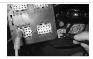
12 - Repair or replace the cable harness.
