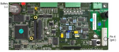
Figure 4-3: Battery Test
