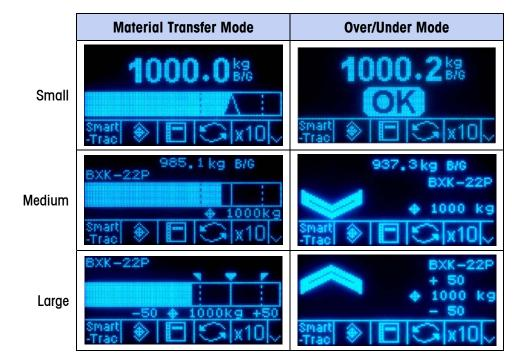
Figure 3-8: SmartTrac Display Sizes, Material Transfer and Over/Under Modes
