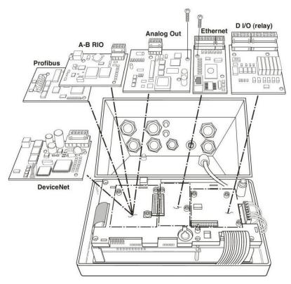
Figure A-22: Option Locations for Harsh Enclosure
