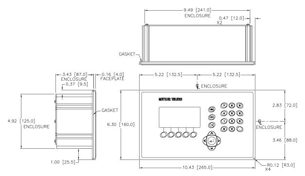
Figure 1-2: IND560 Panel Mount Enclosure Dimensions
