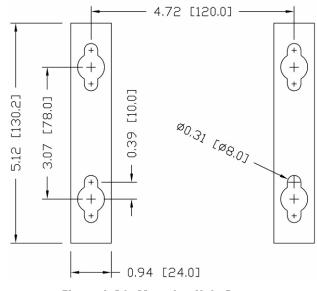
Figure A-10: Mounting Hole Pattern
