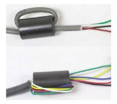
Figure A-11: Installing the Ferrite Cores
