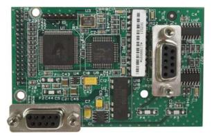
Figure A-39: PROFIBUS Option Board, Harsh Enclosure
