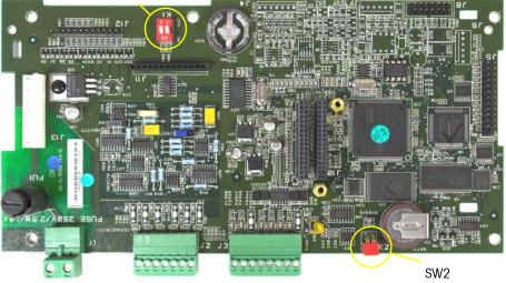
Figure A-43: Main PCB Switches
