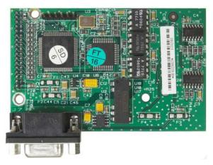
Figure A-41: PROFIBUS Option Board, Panel Mount Enclosure
