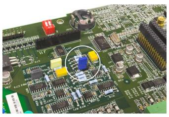
Figure A-45: W1 Millivolt Jumper Location, Main PCB Uncovered
