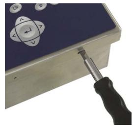
Figure A-2: Opening the Harsh Enclosure
