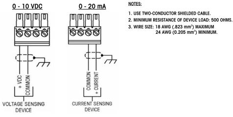
Figure A-25: Wiring the Analog Output
