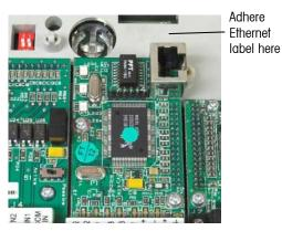
Figure A-29: Ethernet Label Location for the Harsh Enclosure
