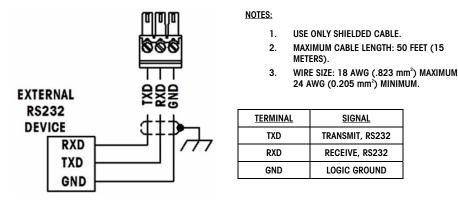
Figure A-27: Wiring to COM2
