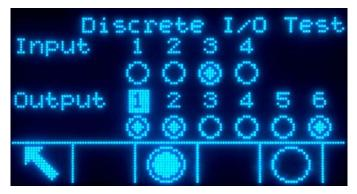
Figure 4-5: Discrete I/O Test Screen
