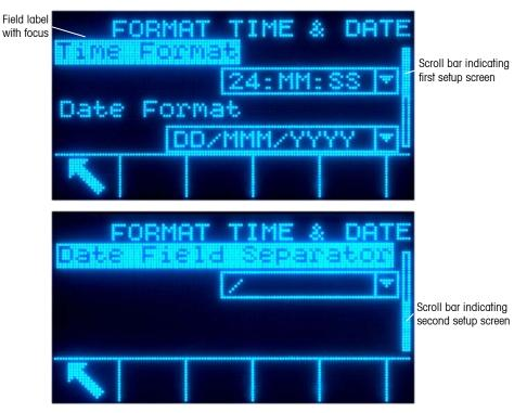
Figure 3-4: Examples of Setup Screens (Format Time & Date)
