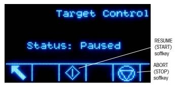
Figure 2-12: Example of Paused State in Target Control
