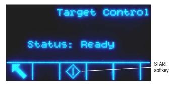
Figure 2-10: Example of Ready State in Target Control
