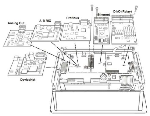
Figure A-23: Option Locations for Panel-Mount Enclosure
