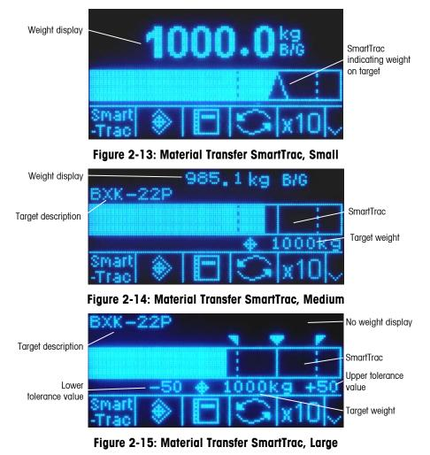
While the bar graph display appears to be one continuous bar graph, it can actually be broken into four separate sections or ranges. Depending upon the target and tolerance values used, there could be one, two, or three speeds at which these graphical sections are filled in. Figure 2-16 illustrates the ranges.
