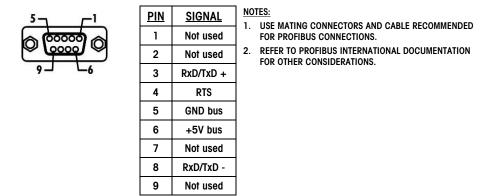
Figure A-42: PROFIBUS Nine-Pin Connector Assignments
