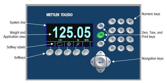
Figure 1-6: The IND560 Front Panel Layout
