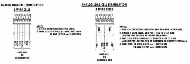
Figure A-16: Load Cell Termination
