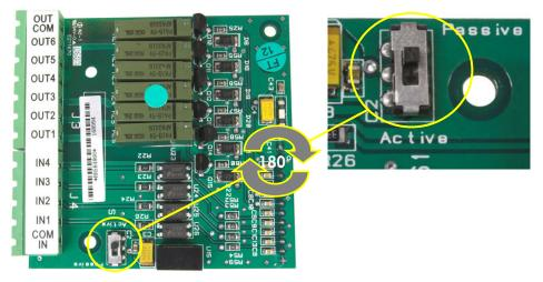
Figure A-44: Location (I) and Switch Settings (r) for Relay Discrete I/O Switch
