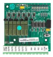
Figure A-30: Discrete I/O Option Board
