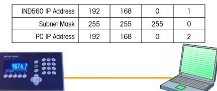
IND560 Setup IP Address: 192.168.0.1 Subnet Mask: 255.255.255.0
