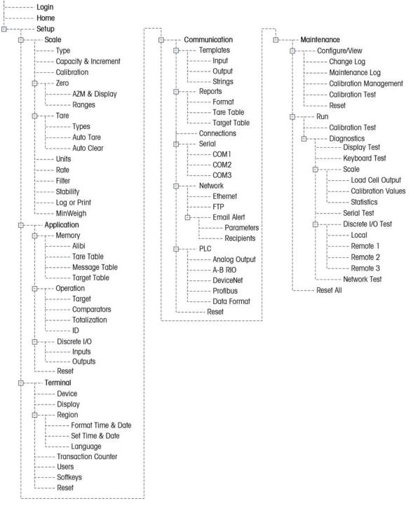
Details for each branch are provided in the following Configuration Options section. Figure 3-6 shows the setup menu tree with all branches expanded.
