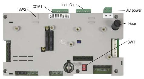
Figure A-14: Analog Main Board in Harsh Enclosure
