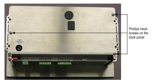
Figure A-1: Opening the Panel-Mount Enclosure
