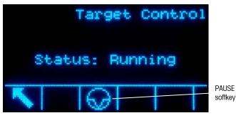
Figure 2-11: Example of Running State in Target Control
