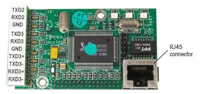
Figure A-26: Ethernet Connection Option Board
