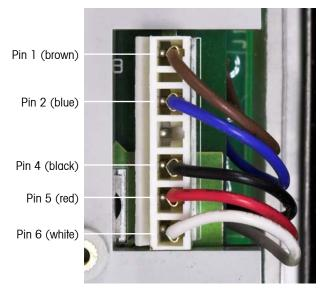
Figure 4-2: Pin Locations on the Power Supply Harness
