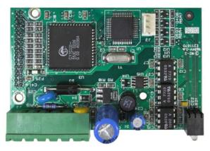
Figure A-36: DeviceNet Option Board
