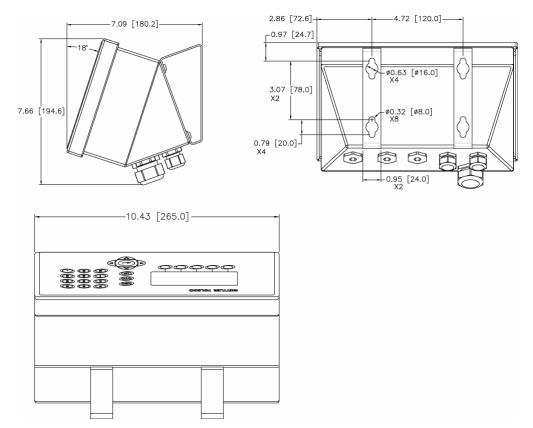
Figure 1-5: Harsh Environment Enclosure Dimensions with Optional Brackets
