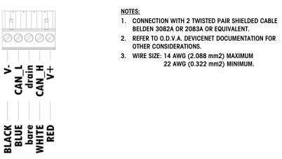
Figure A-38: DeviceNet Connector Wiring
