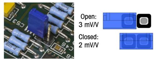
Figure A-47: W1 Millivolt Jumper Settings
