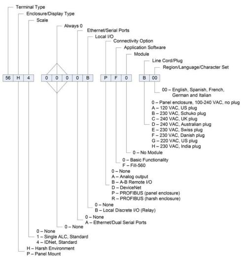
Figure 1-1: IND560 Model Identification Numbers
