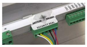
Figure A-58: Analog Load Cell Paper Seal
