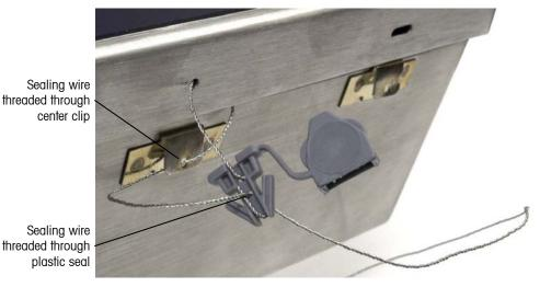
Figure A-53: Harsh Enclosure Seal Threaded and Ready to be Closed
