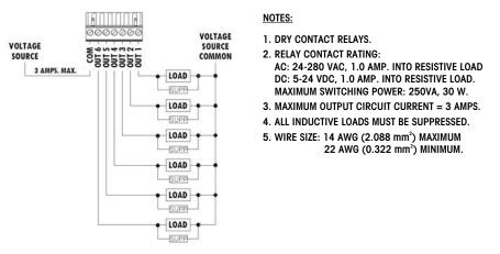
Figure A-33: Relay Outputs
