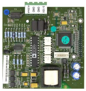
Figure A-24: Analog Output Option Board
