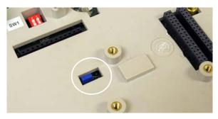
Figure A-46: W1 Millivolt Jumper Location, Main PCB Cover Installed
