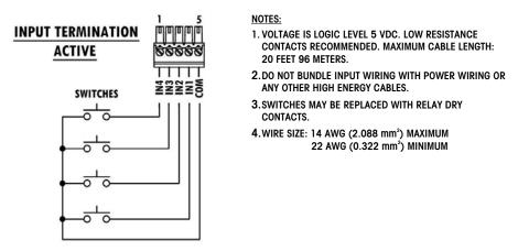
Figure A-31: Active Input Connections
