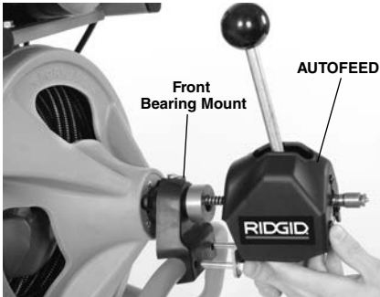
Figure 5 – Mounting AUTOFEED onto the Frame
