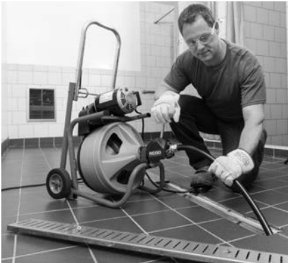
Figure 16 – Using Machine with Guide Hose
