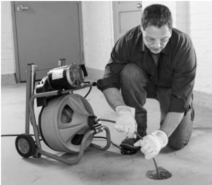
Figure 13 – In Operating Position, Manually Feeding Cable
