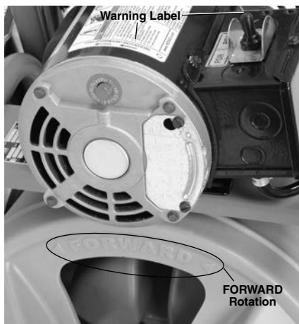
Figure 8 – Proper Drum Rotation (FOR Switch Position)
