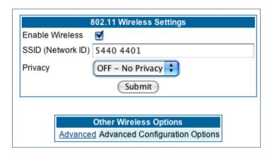
If you uncheck the **Enable Wireless** checkbox, the Wireless Options are disabled, and the Gateway will not provide or broadcast any wireless LAN services.
