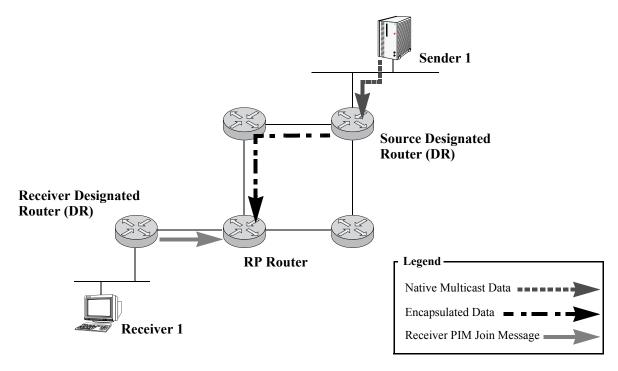
Once the distribution tree for group G is learned at the RP, the encapsulated data being sent from the source DR are now unencapsulated at the RP and forwarded natively to the Receiver.
