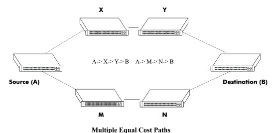
Delivery of packets along equal paths is based on flows rather than a round-robin scheme. Equal cost is determined based on standard routing metrics. However, other variables, such as line speed, are not considered. So it is possible for OSPF to decide two paths have an equal cost even though one may contain faster links than another.
