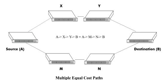
Delivery of packets along equal paths is based on flows rather than a round-robin scheme. Equal cost is determined based on standard routing metrics. However, other variables, such as line speed, are not considered. So it is possible for OSPFv3 to decide two paths have an equal cost even though one may contain faster links than another.
