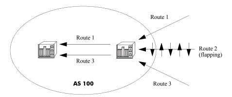
Routes 1, 2, and 3 are entering AS 100, but Route 2 (because it is flapping) has exceeded the dampening threshold. It is therefore not propagated into the AS.
