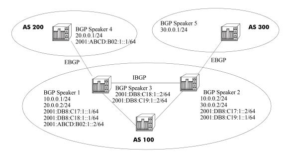
In the above network, Speakers 1, 2, and 3 are part of AS 100 and are fully meshed. Speaker 4 is in AS 200. Speaker 3 is part of a homogenous IPv6 network domain (i.e. pure IPv6 network), internal to AS 100. Speaker 5 in AS 300 is not aware of IPv6 capabilities.
