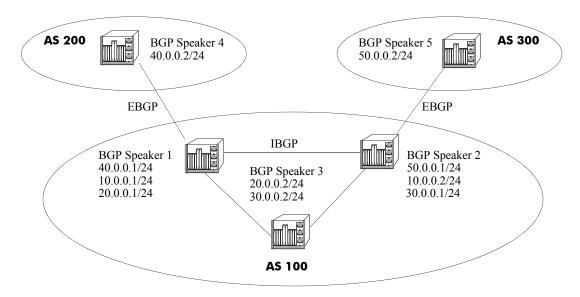
In the above network, Speakers 1, 2, and 3 are part of AS 100 and are fully meshed. Speaker 4 is in AS 200 and Speaker 5 is in AS 300.
