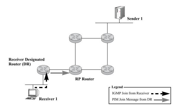
**Note.** Depending on the network configuration, multiple routers may exist between the receiver's DR and the RP router. In this case, the (\*, G) Join message travels hop-by-hop toward the RP. In each router along the way, the multicast tree state for group G is instantiated. These Join messages converge on the RP to form a distribution tree for group G that is rooted at the RP.
