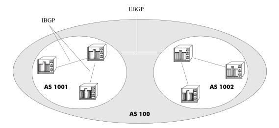
AS 100 is now a confederation consisting of AS 1001 and AS 1002. Even though EBGP is used to communicate between AS 1001 and 1002, the entire confederation behaves as though it were using IBGP. In other words, the sub AS attributes are preserved when crossing the sub AS boundaries.
