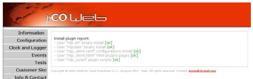
Figure 9.p – "NTP" Plugin installation report
