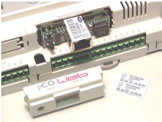
Figure 2.c – Inserting pCOWeb in the pCO controller
