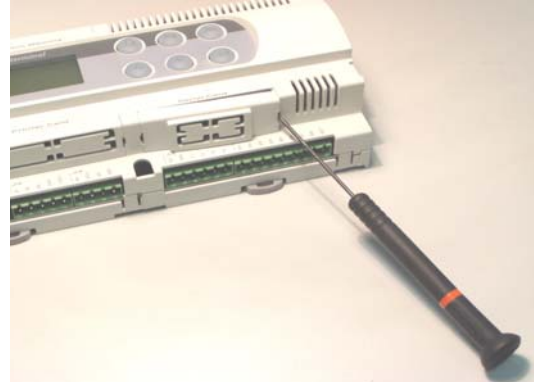
Figure 2.b – Removing the cover from the pCO controller
