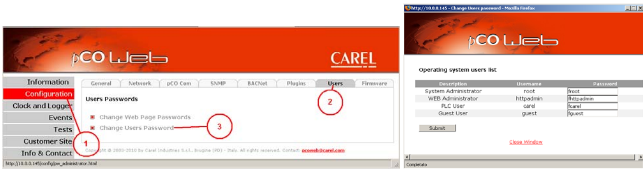
Figure 9.x – Changing the password for the operating system access Usernames
