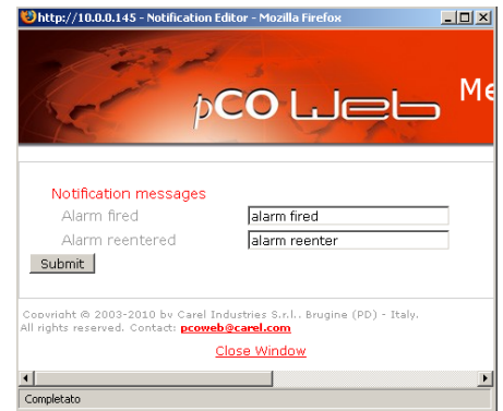
Figure 4.r – Setting the strings sent for Activation - Return
