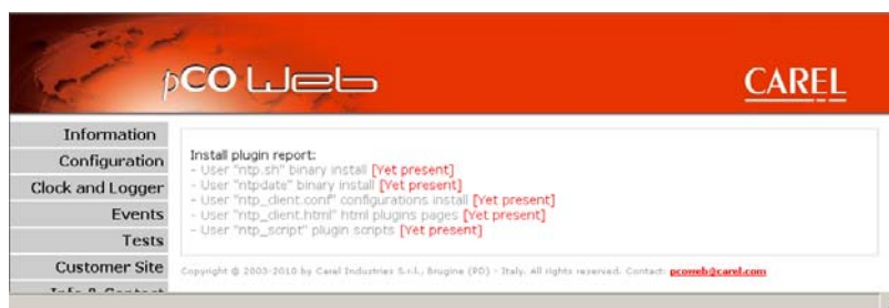
Figure 9.q – “NTP” Plugin installation report if the Plugin is already installed
