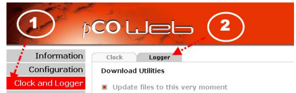
Figure 5.c - Opening the Logger and Graph settings
