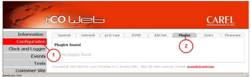
Figure 9.m - Installing / uninstalling the Plugins
