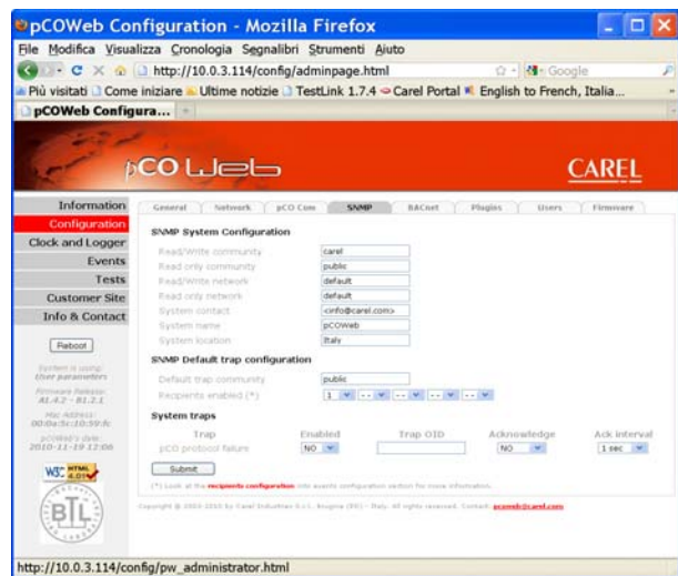
Figure 6.b - SNMP: basic configurations
