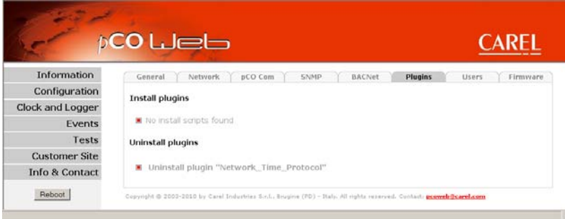
Figure 9.t – Install/Uninstall Plugin page after having installed "NTP"
