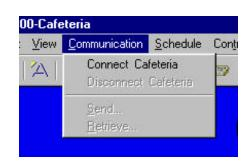
2. Click on Connect. You will see a message telling you that the software is attempting to connect to the character generator. When the connection is successful, you will receive confirmation about the connection. The connection will be made according to the instructions you gave when you originally set up the channel. I.e. if your connection is via a modern, then the remote telephone number will be dialed automatically.
