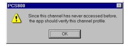
Clicking OK then lets the software interrogate the remote character generator and get the data contents, if any, into the computers memory. This synchronizes the computer with any data that might have been changed by another user in that particular character generator.
