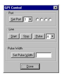
to the selected line A pulse is defined as taking the line to the opposite state that it is currently in for the duration of the pulse width
