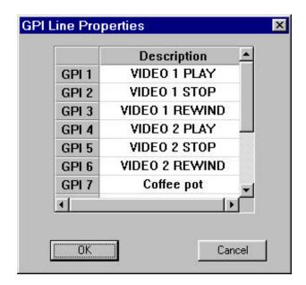
The first thing you must do is establish that the control lines are initialized to their off state. In the case where the line must pulse from HIGH to LOW then the OFF state is HIGH.
