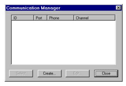
dialog box. You must set up the parameters for the serial port connection to the remote 840AE character generator. Click on Create and you will see the following:
