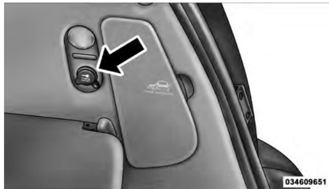
Rear Power Outlet
