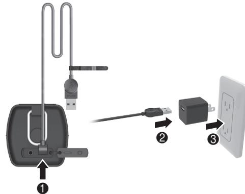
It is recommended to fully charge the battery before first time use. First time charging will take approximately 2-3 hours. The Power button light flashes white while charging and stops flashing once charging is complete.
