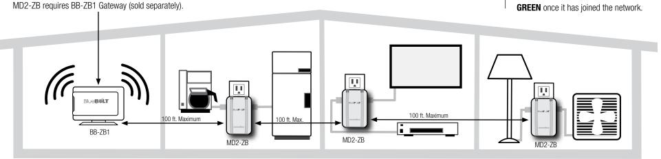
Multiple MD2-ZB units can be installed within 100 ft. from an active device (BB-ZB1 or another active MD2-ZB).
