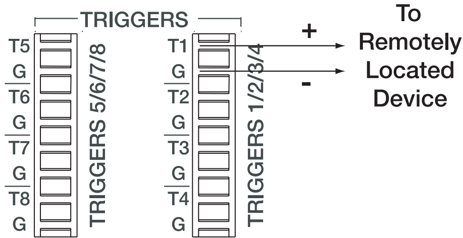
Figure 3-13: Programmable Trigger Connections
