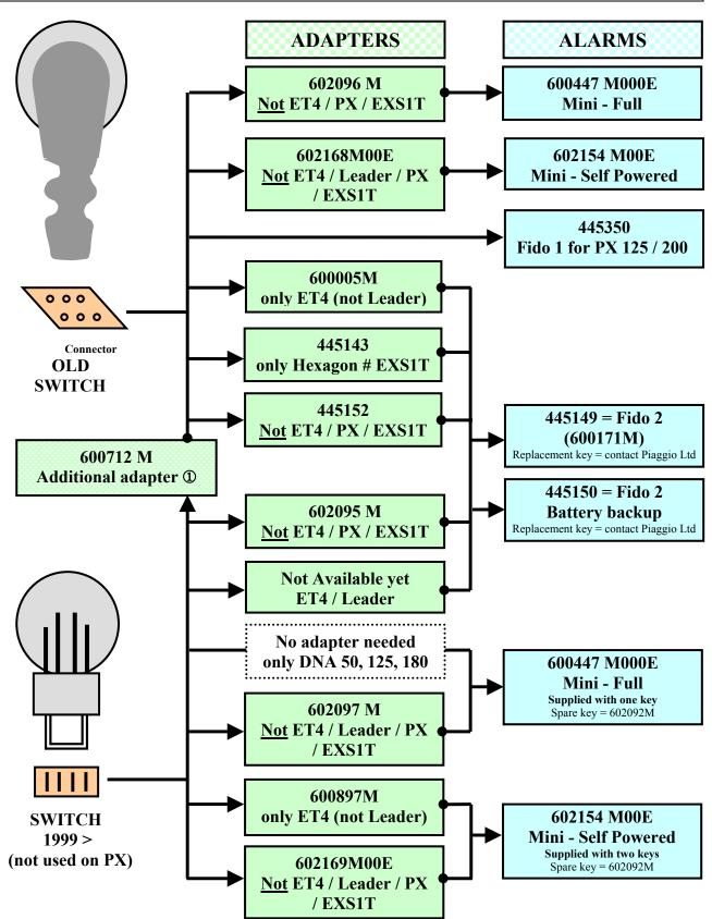
The new LEADER engine has a very different electrical system and an adapter for this is not available yet. **Do not** try to use any existing adapter.
