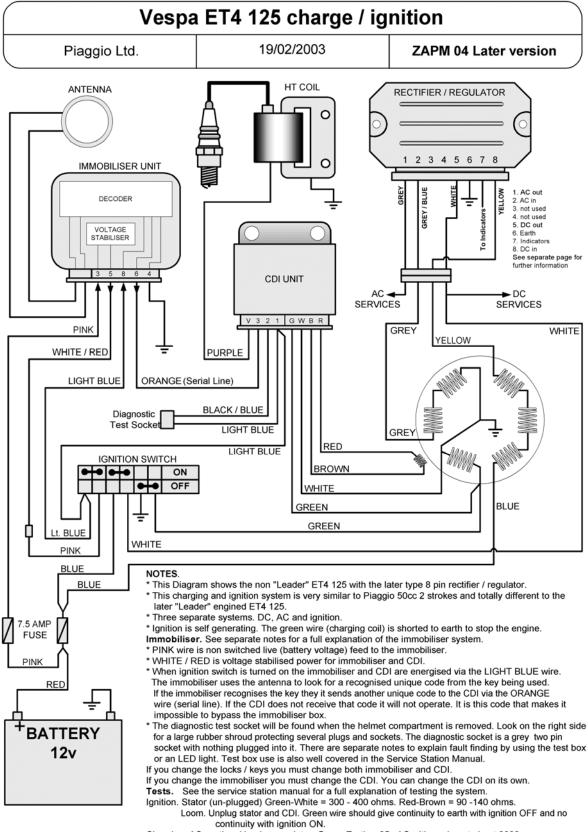
Charging. AC section. Un-plug regulator. Grey - Earth = 25v AC with engine at about 3000 rpm. DC section. Ammeter between Battery + and red wire = at least 1.8 amps, fully charged battery
