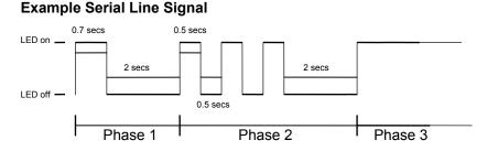
The above diagram shows the trace of the diagnostic signal for Decoder and CDI Units both programmed, using a key with an unknown transponder (Table 2, case 5), resulting in 3 FLASHES during the second phase of the diagnostic signal (Phase 2).
