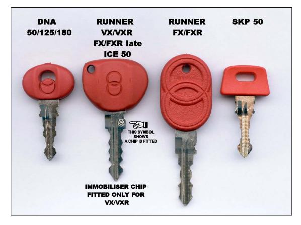
Only the Runner VX / VXR has an immobiliser. Note the symbol on the key that denotes an immobiliser chip is fitted.
