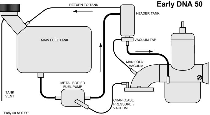
1. Carburettor is gravity fed not pressure fed.
