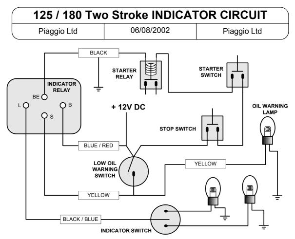
ABOVE. Vehicles 1999> Cirduit with oil check light that comes on when ignition is switched on.
