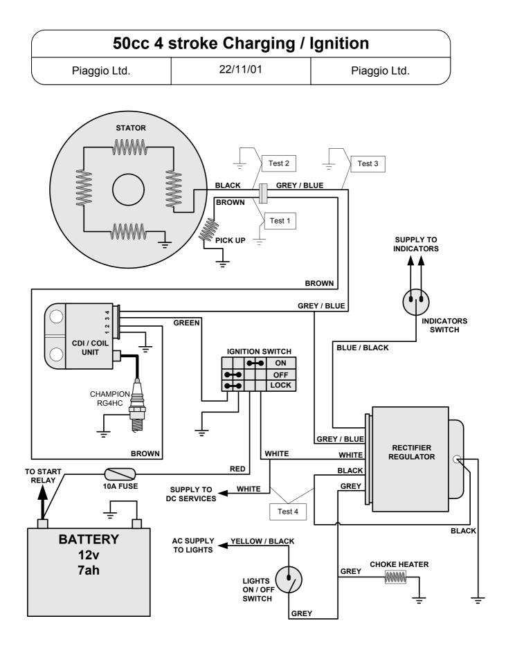
Only two wires come from the stator. The engine to earth connection is very important.
