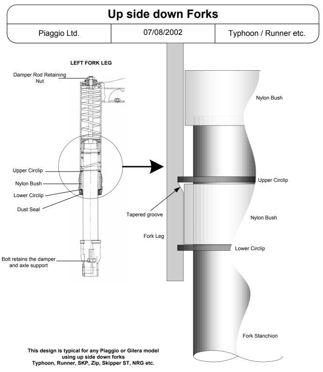
Forks are grease filled for lubrication. The grease can be expected to work past the nylon bush so the chrome stanchion will get a dirty ring round it.
