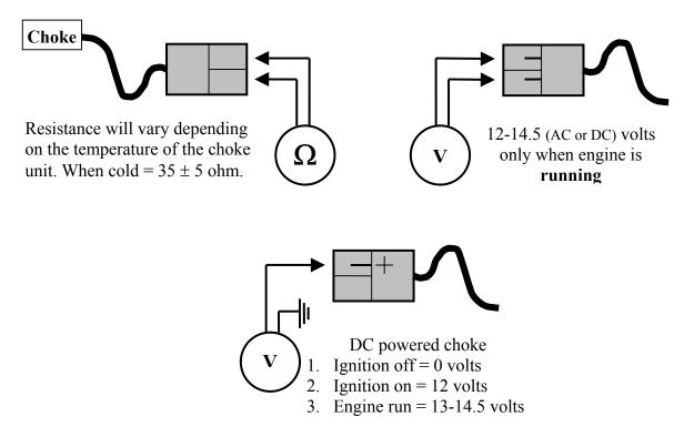
**Note**. Choke units all look much the same but are different and it is important to use the correct choke in the correct carburettor.
