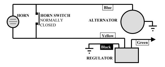
The T5 has a very simple 12 volt AC electrical system but one thing may not be clear when you look at the wiring diagram.
