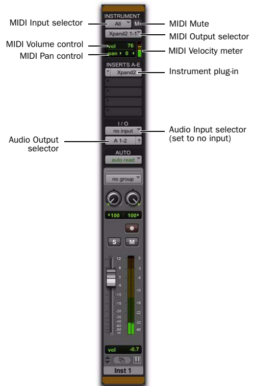
Instrument track configured to control and monitor an instrument plug-in (Xpand 2 shown)
