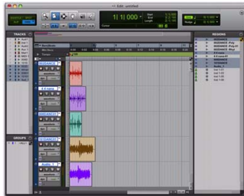
New tracks after dropping multiple Region List items, with Timeline Drop Order set to Top to Bottom mode
