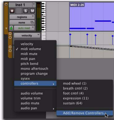
Selecting Add/Remove Controllers from the Controller Type selector on a Controller lane
