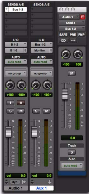
New Auxiliary Input track with audio track send automatically assigned to Bus 1-2
