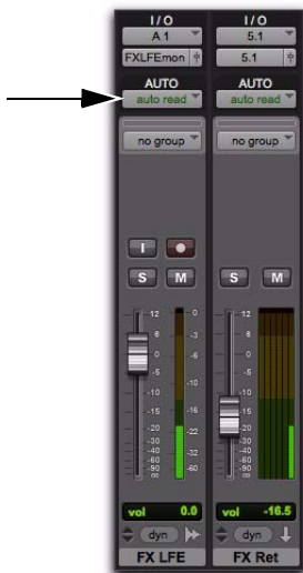
Discrete LFE routing, with main output to mono LFE channel
