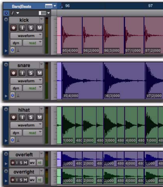
Figure 9. Overhead mic track displaying a collection of beat triggers containing unique triggers generated from the kick, snare, and hi-hat tracks
