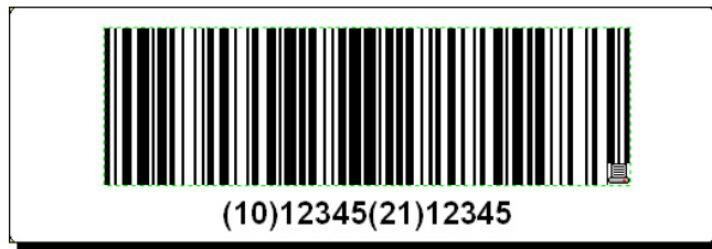
The designed label with EAN.UCC 128 bar code
