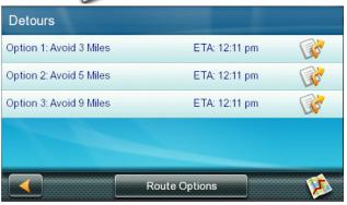
Different detours are calculated using the same routing method that was used to create the route. The list of alternate routes is displayed.
