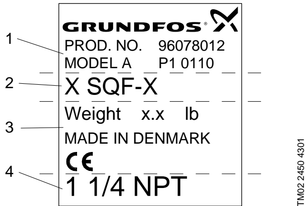
Fig. 1 Example of nameplate, helical rotor pump
