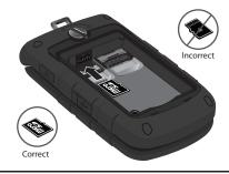
**Warning!:** Please note the printed circuit side faces down when inserting the card.
