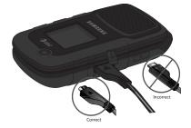
Note: The previous illustration is the correct and incorrect method for connecting the charger. If the incorrect method is attempted, damage to the accessory port will occur therefore voiding the phone's warranty.
