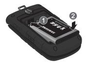
With the battery in position on the phone, place the cover back on the handset (1) then press down firmly (2). Press down along the edges to make sure the cover is flush with the phone and that there is a tight seal. 4. Turn the grooved dial clockwise until the cover locks.
