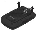
3. Lift the battery up (1) and away (2) from the phone, as shown.
