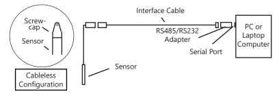
Connect the sensor to your computer using an RS485/RS232 adapter and an interface cable.
