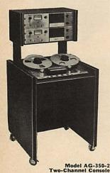
Tape Speeds: 7½ and 15 lps, or 3¾ and 7½ lps. Tape Width: Standard ¼ tape. Reel Size: 10½ max. Overall Frequency Response: ±2 db, 30-18,000 cps at 15 lps; ±2 db, 40-10,000 cps (+2, -4 db, 30-15,000 cps) at 7½ lps; ±2 db, 50-7,500 cps at 3½ lps. Flutter (ASA Z57.1-1954 standard): Below 0.11% rms at 15 lps; 0.14% rms at 7½ lps; 5.19% rms at 3½ lps. O.18% rms at 3½ l
